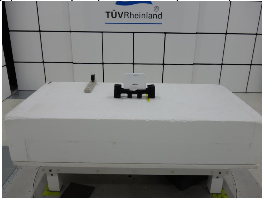
Photograph 8: Test Setup for Spurious Emissions (Front View 2)
