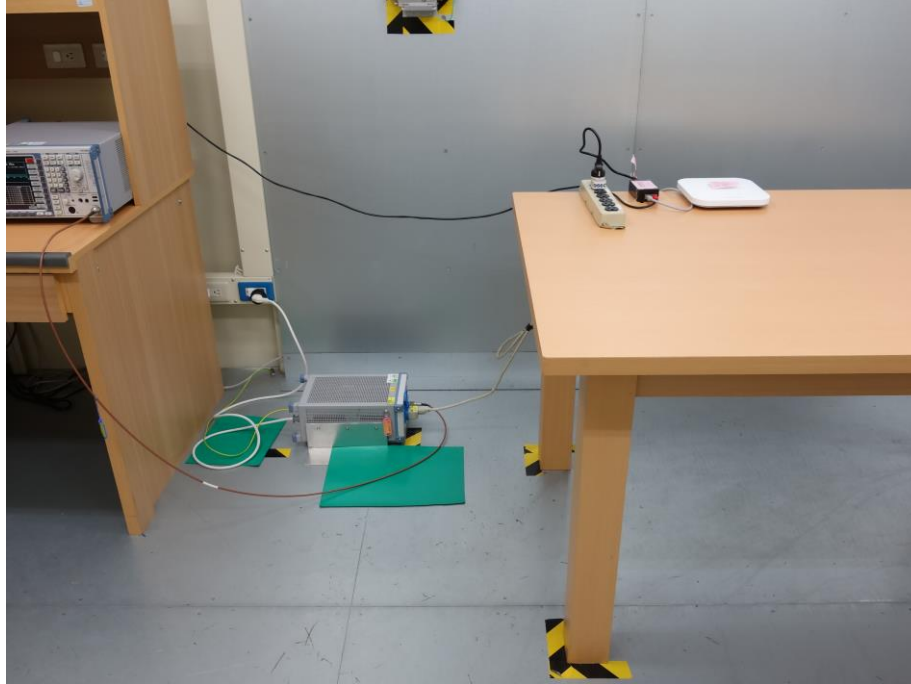
Photograph 19: Test Setup for Mains Conducted Emissions (Front View)
