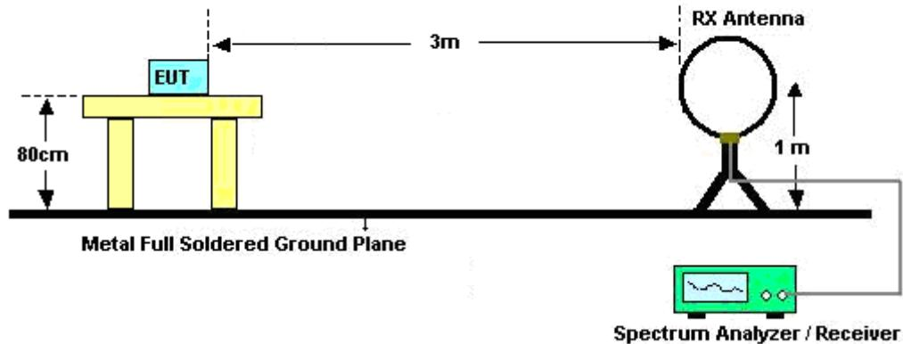
For radiated emissions from 30MHz to 1GHz
