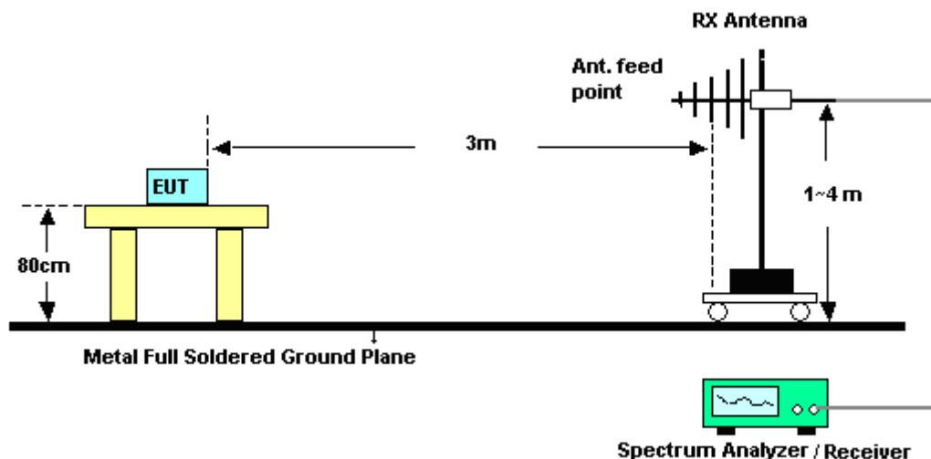
**For radiated emissions above 1GHz**
