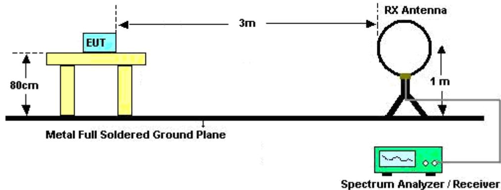
For radiated emissions from 30MHz to 1GHz
