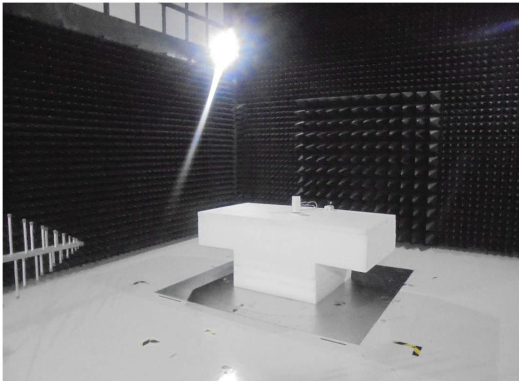
**Radiated Emission Above 1GHz Test**
