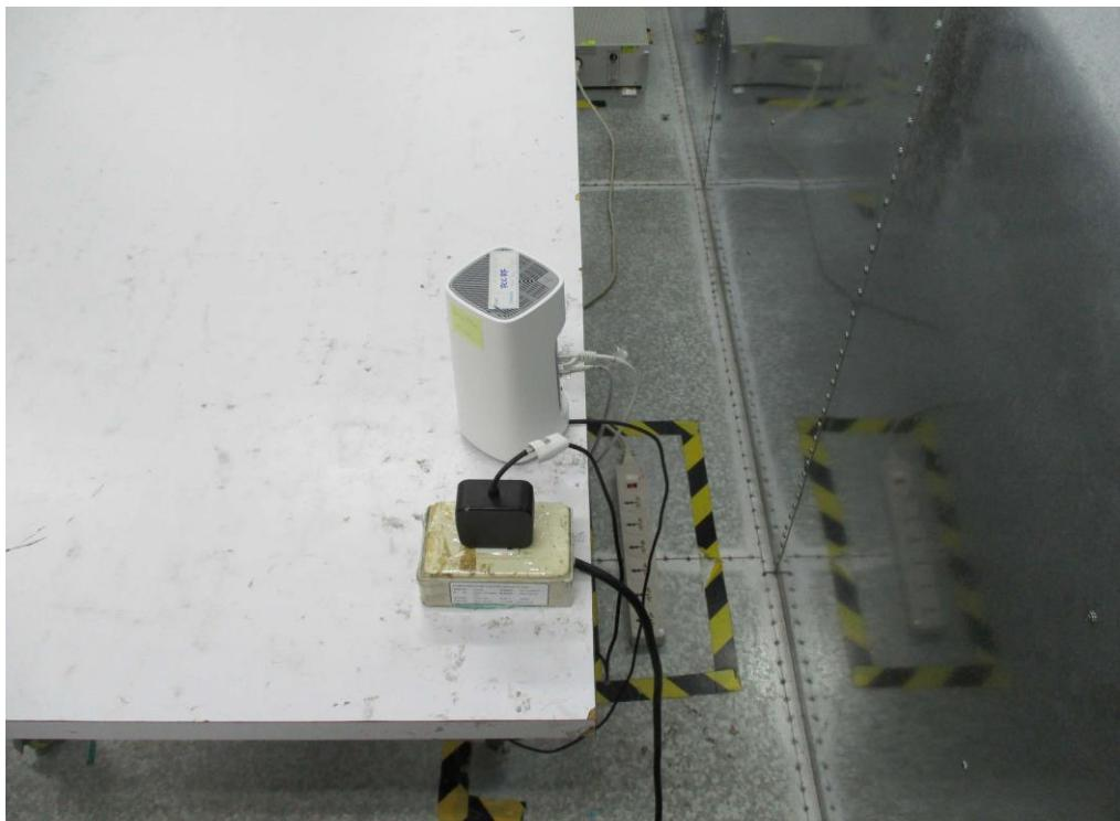
**Radiated Emission Below 1GHz Test**
