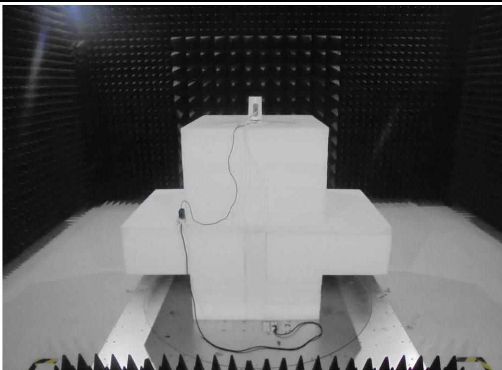
**Radiated Emission Above 1GHz Test**
