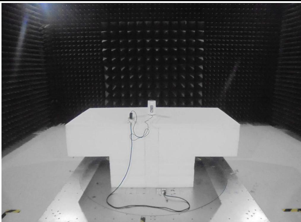
**Radiated Emission Below 1GHz Test**
