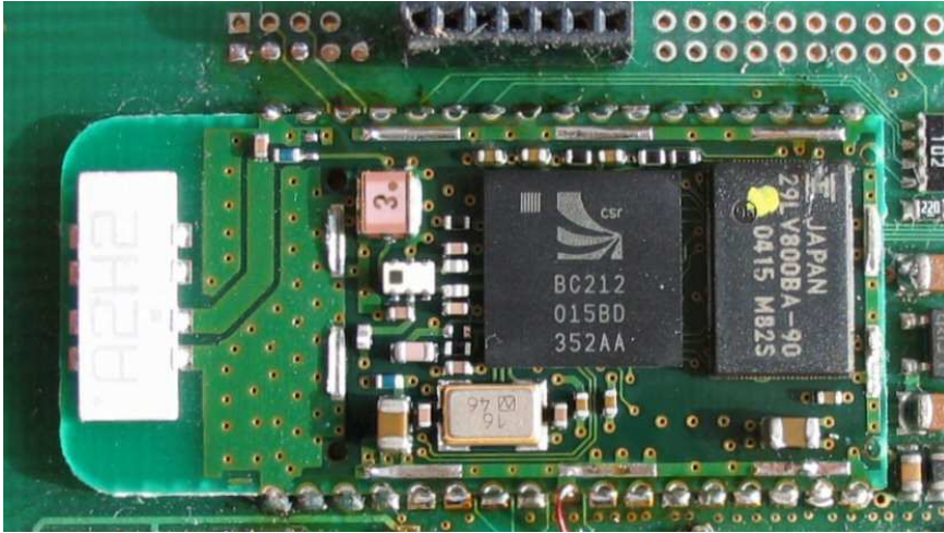
Open Bluetooth module with antenna
