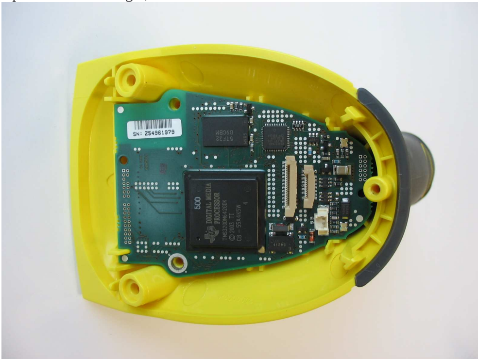
Main board 6320 top side
