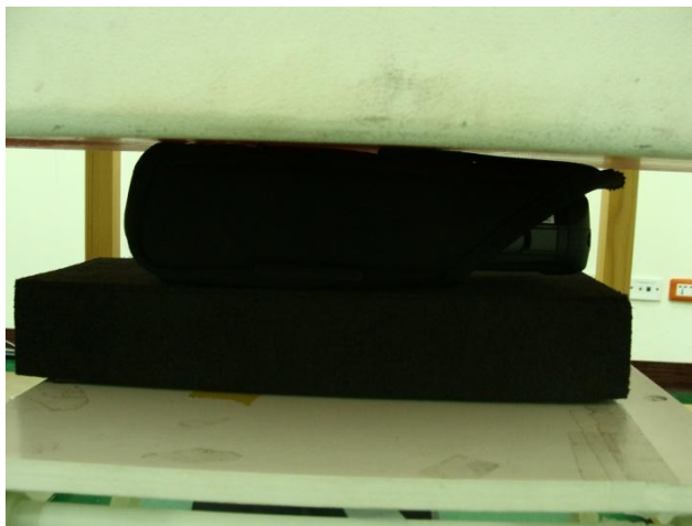
Bottom of the DUT and Holster with Phantom 0 cm Gap
