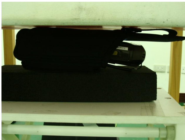
Face of the DUT and Holster 2 with Phantom 0 cm Gap (DUT with Keypad 4)
