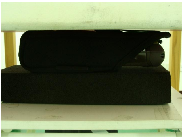
Bottom of the DUT and Holster 1 with Phantom 0 cm Gap (DUT with Keypad 4)
