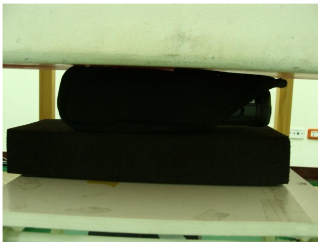
Bottom of the DUT and Holster 1 with Phantom 0 cm Gap (DUT with Keypad 1)
