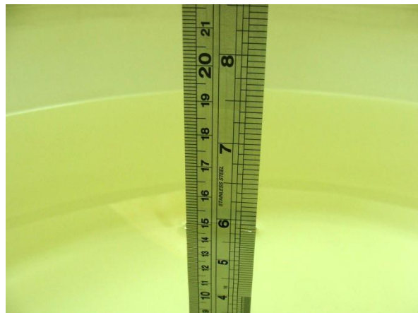
Fig 6.2 Photo of Liquid Height for Body SAR
