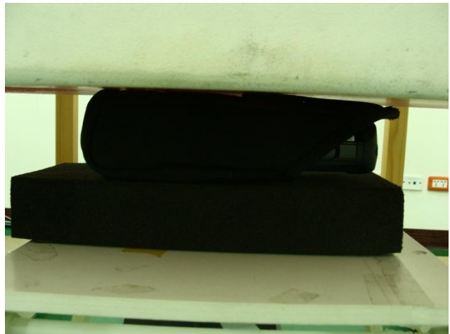
Bottom of the DUT and Holster with Phantom 0 cm Gap
