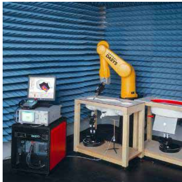
Fig. 5.2 Probe Setup on Robot
