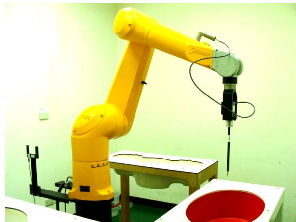
Fig 5.8 Photo of DASY5
