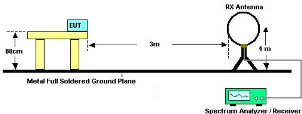
For radiated emissions from 30MHz to 1GHz
