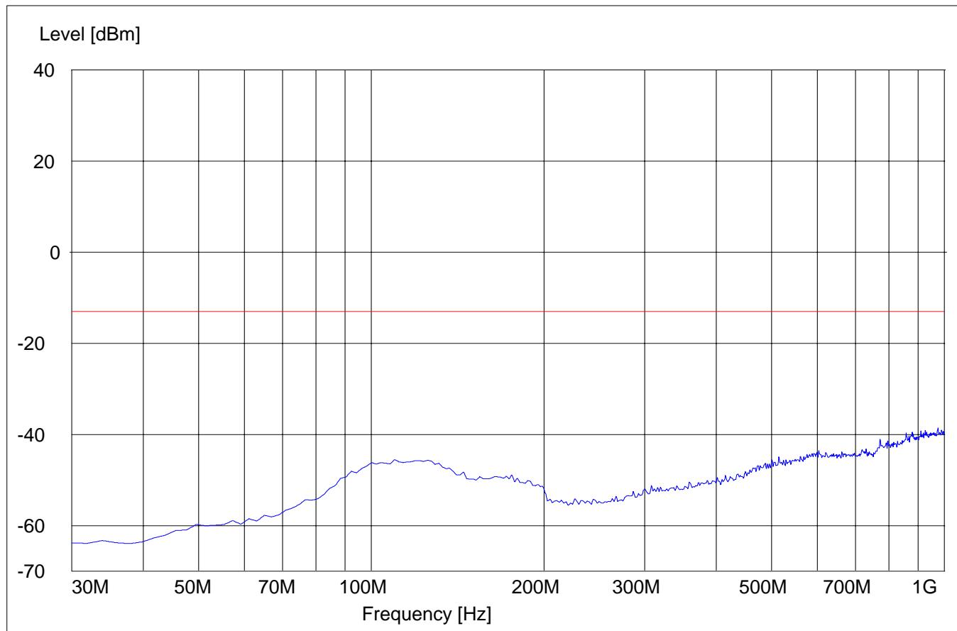
**RADIATED SPURIOUS EMISSIONS****30MHz - 1GHz**
