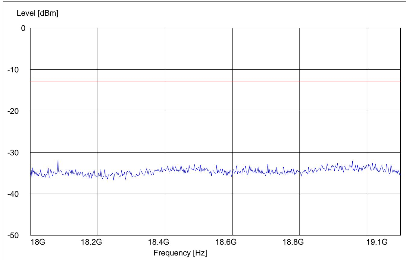
**COLLOCATION BT & GSM:****EMISSION LIMITATIONS - Radiated (Transmitter)**
