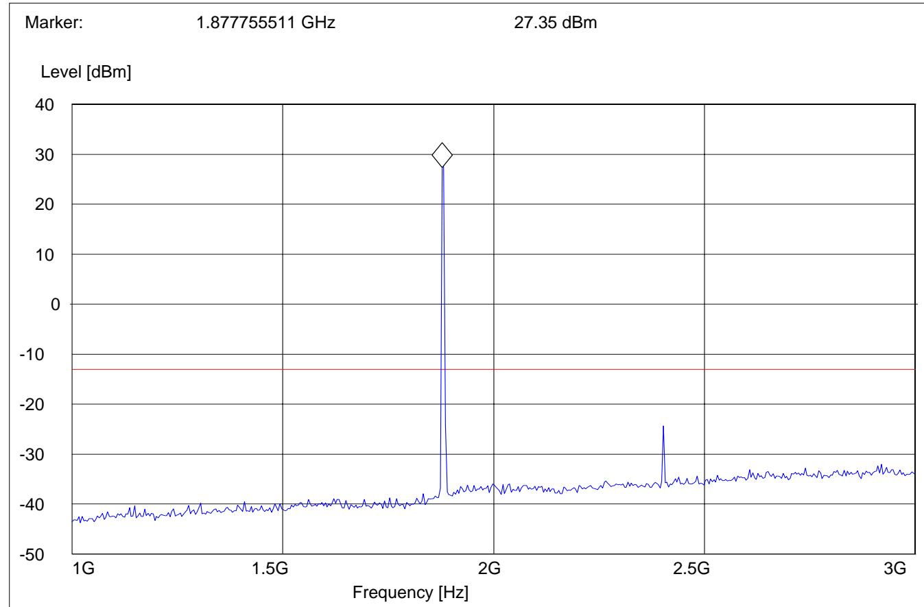
**EMISSION LIMITATIONS - Radiated (Transmitter)****§ 15.247 (c) (1)****3-18GHz****BT Tx @ 2441MHz****GSM Tx @ 1880MHz**
