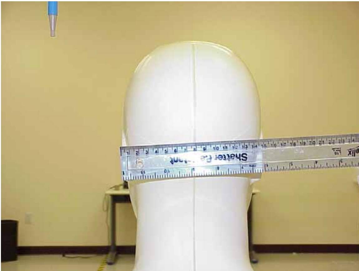
Photo 9. Photo to demonstrate 15 cm Z-axis head phantom
