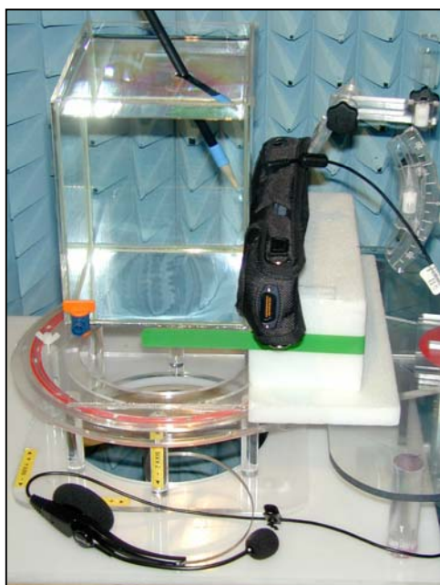
Figure 43. A Positional photograph of the D9500 Device Fitted with Normal Battery positioned Rear Facing 0.0mm from the Flat Phantom
