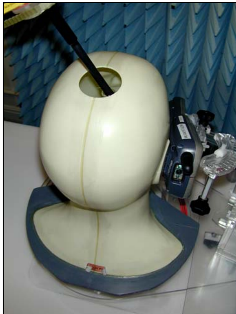
Figure 41. Positional photograph of D9500 Device in the Right-hand Cheek Position
