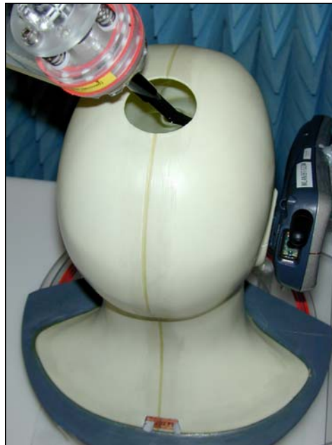
Figure 42. Positional photograph of D9500 Device in the Right-hand 15 Degree Position
