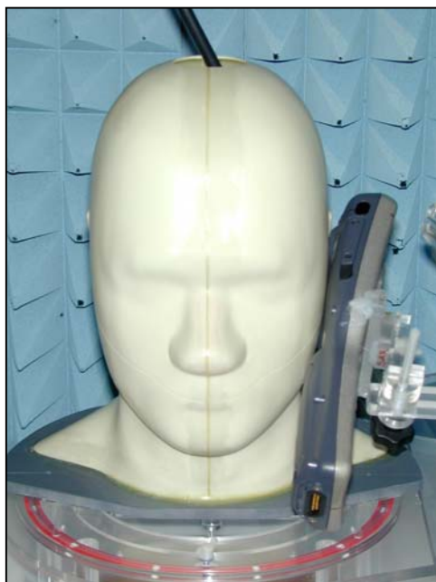
Figure 39. Positional photograph of the D9500 Device in the Left-hand Cheek Position
