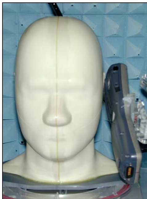
Figure 40. Positional photograph of D9500 Device in the Left-hand 15 Degree Position
