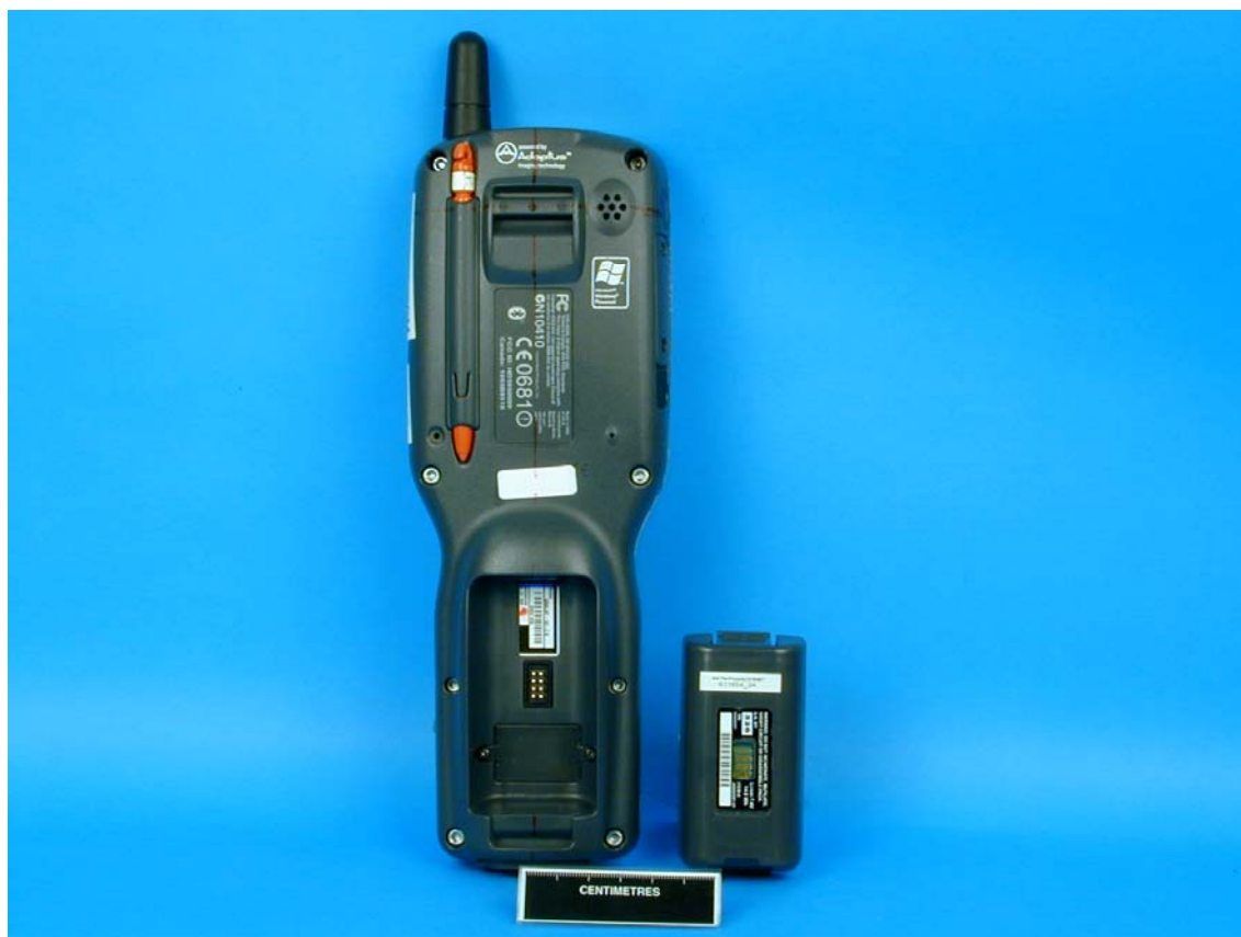
Figure 47. Rear view of the HHP D9500 Device with battery removed.
