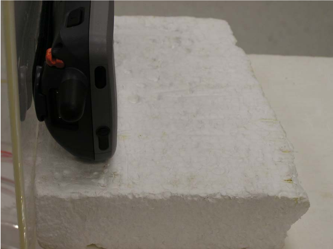
Photo 7 Belt clip touching phantom.
