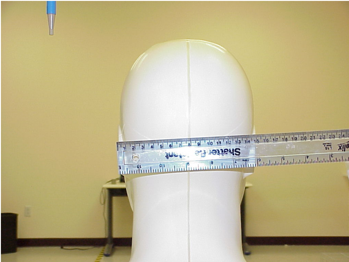
Photo 8. Photo to demonstrate 15 cm Z-axis head phantom
