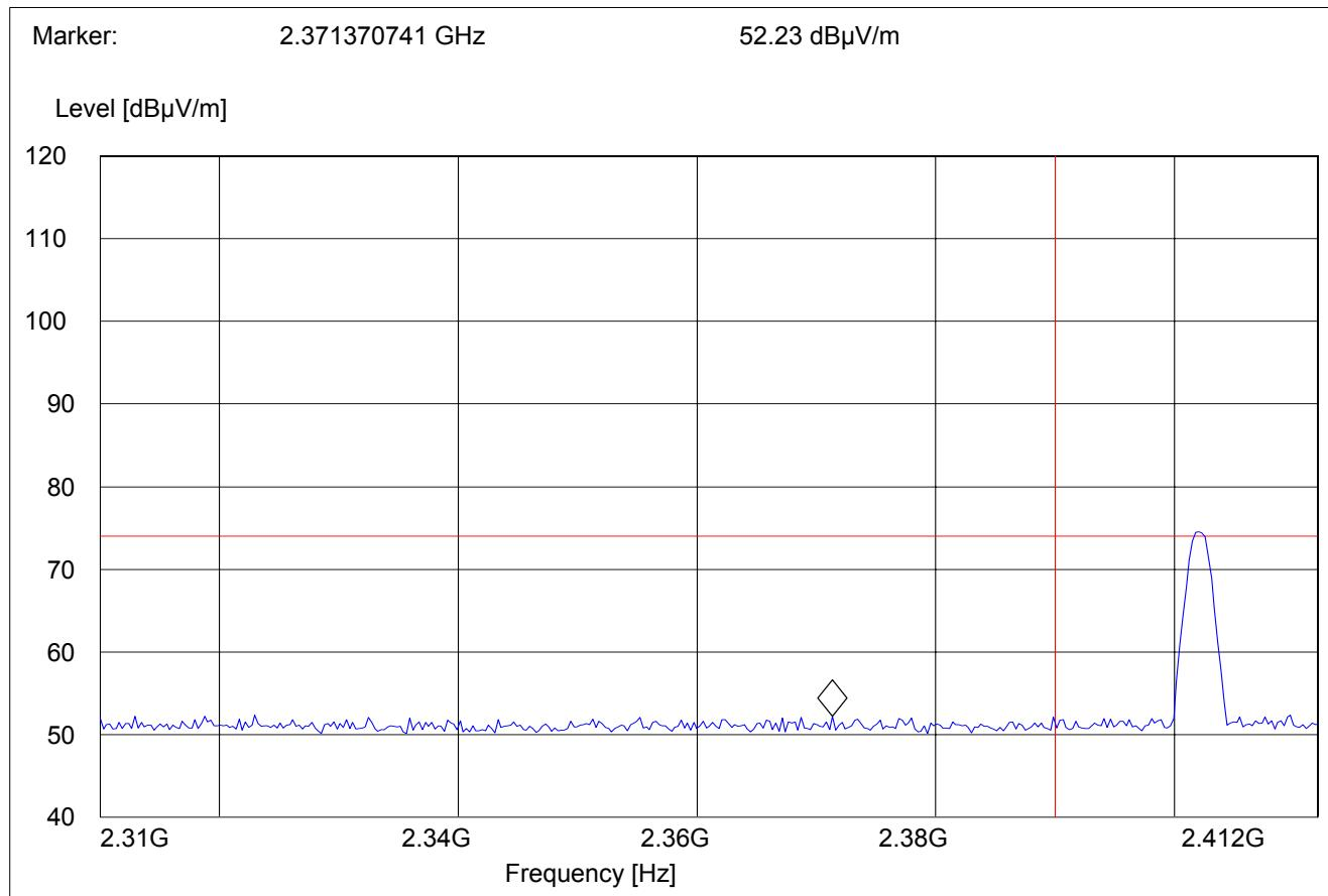
**BAND EDGE COMPLIANCE****§15.247 (c)****High frequency section (spurious in the restricted band 2483.5 – 2500 MHz)****Average Measurement****(This plot is valid for both Hopping ON & OFF)**
