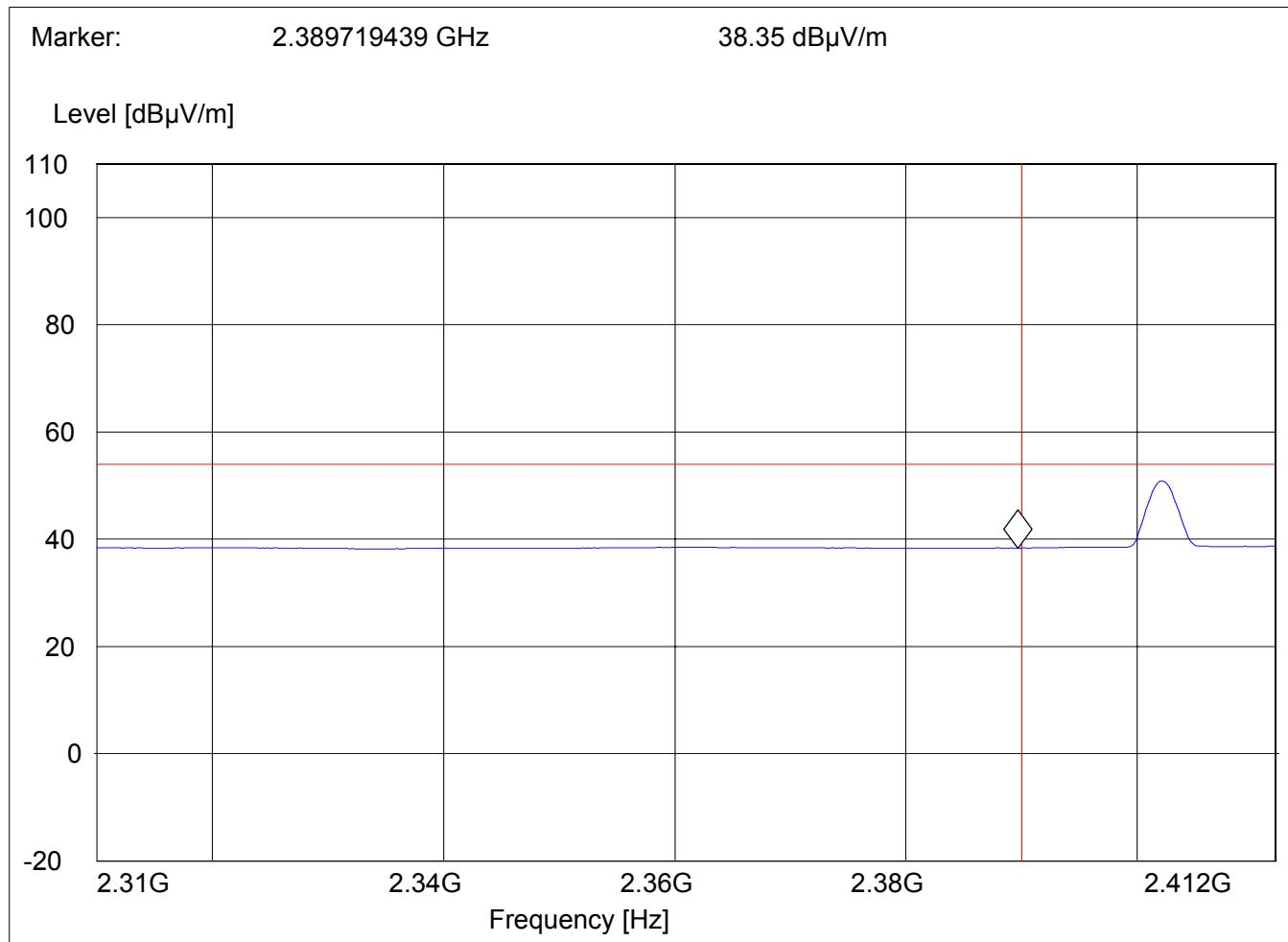
**BAND EDGE COMPLIANCE****§15.247 (c)****Low frequency section (spurious in the restricted band 2310 – 2390 MHz)****Peak Measurement****(This plot is valid for both Hopping ON & OFF)**
