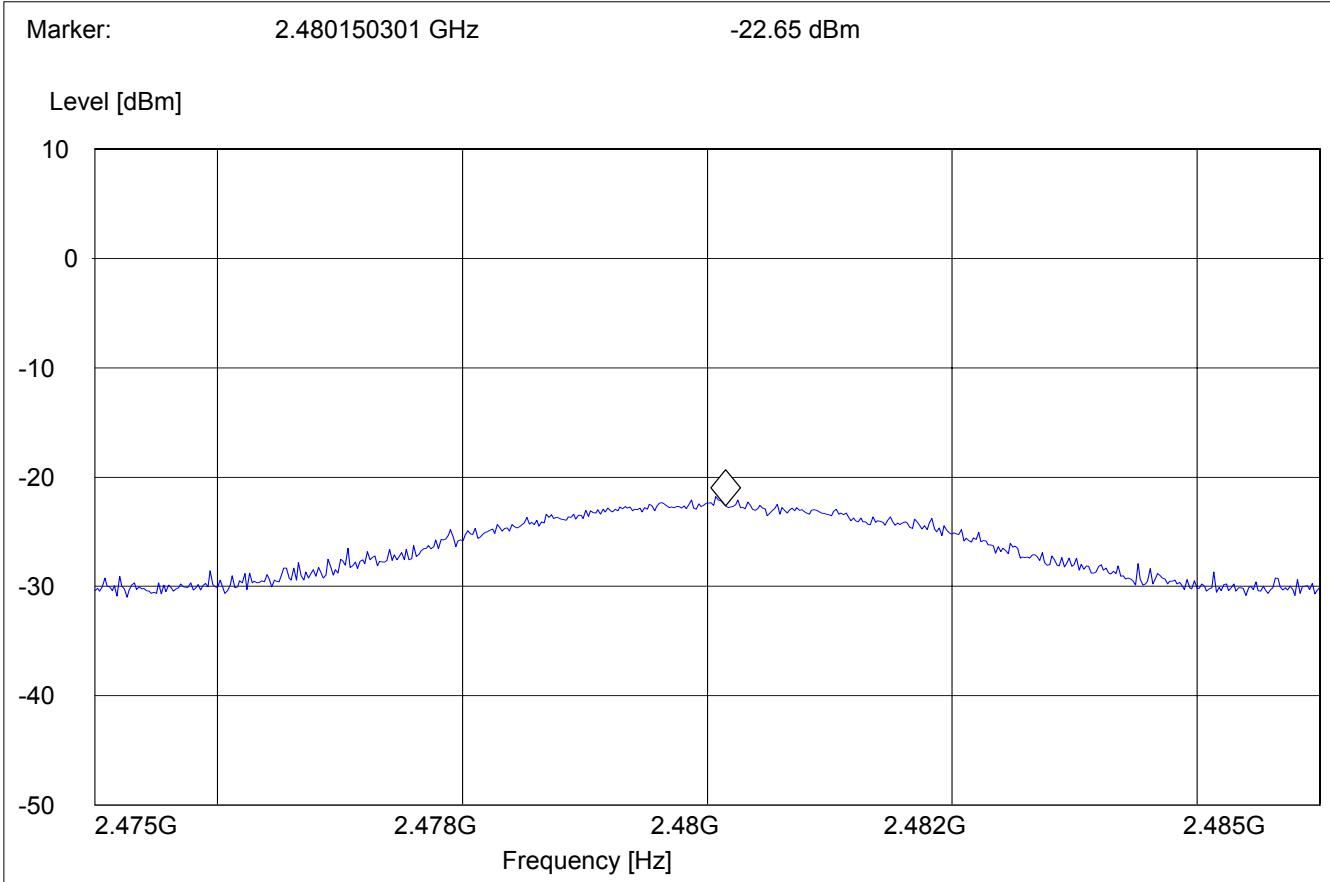
**BAND EDGE COMPLIANCE****§15.247 (c)****Low frequency section (spurious in the restricted band 2310 – 2390 MHz)****Average Measurement****(This plot is valid for both Hopping ON & OFF)**
