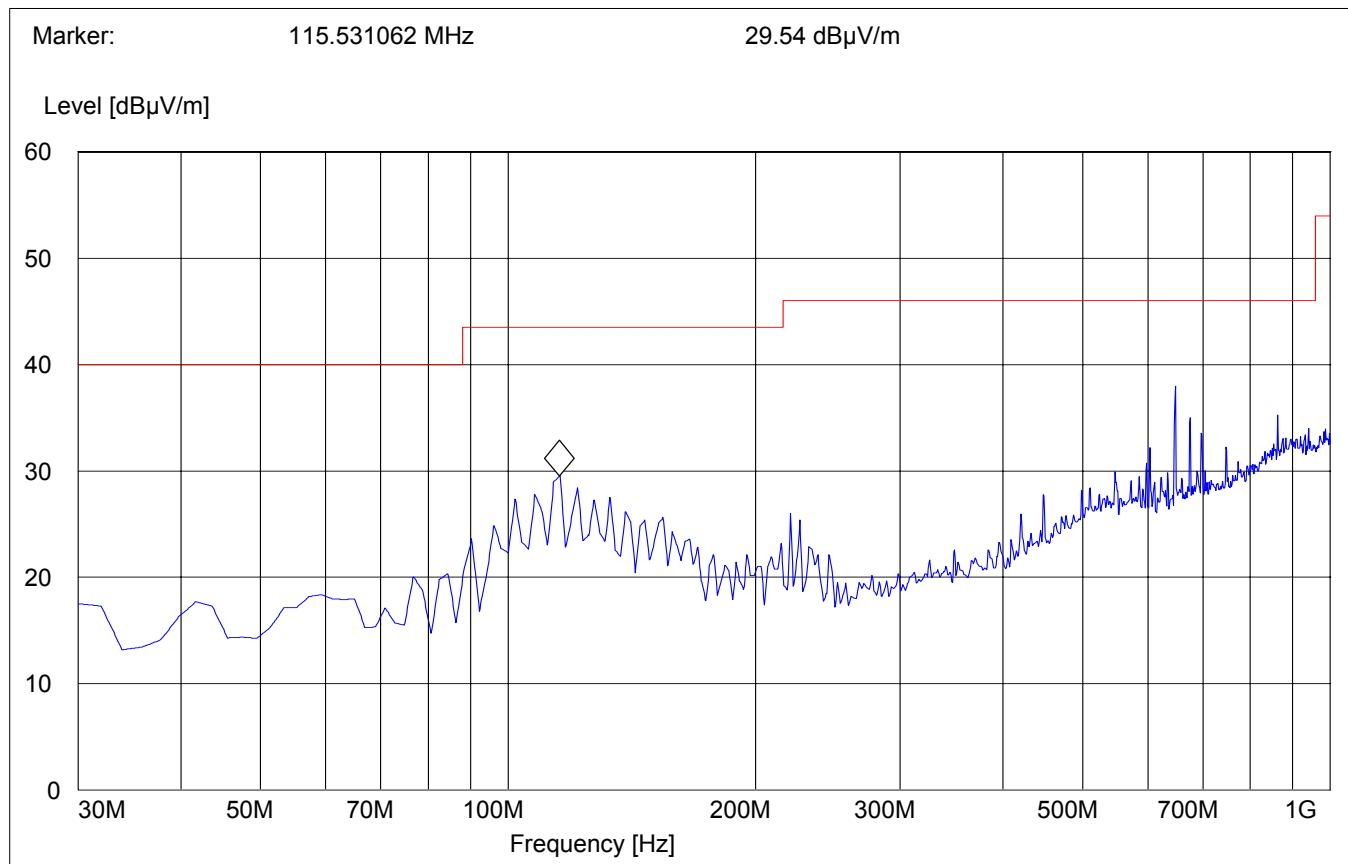
**EMISSION LIMITATIONS - Radiated (Transmitter)****§ 15.247 (c) (1)****30MHz – 1GHz****Antenna: horizontal****Note: This plot is valid for low, mid & high channels (worst-case plot)**
