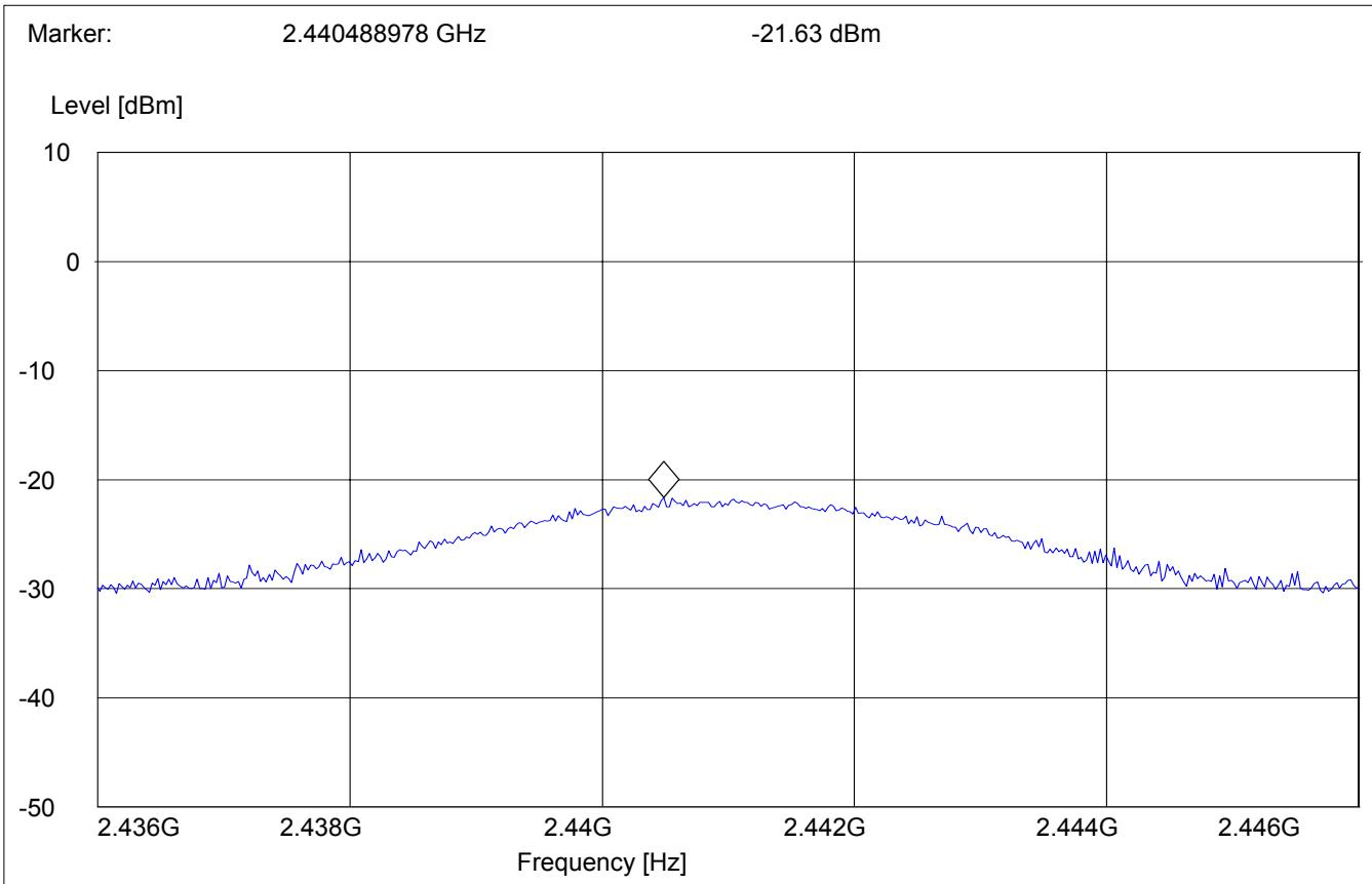
**PEAK OUTPUT POWER (RADIATED)****§15.247 (b) (1)****Highest Channel:** Error! Reference source not found. **MHz**
