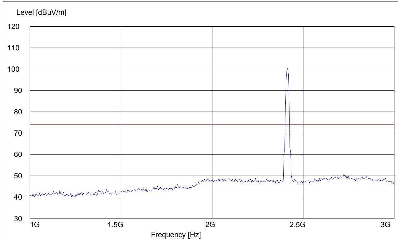
**EMISSION LIMITATIONS - Radiated (Transmitter)****§ 15.247 (c) (1)****Operating Mode: BT @ CH 0 + WLAN @ CH 1****Average Measurement**
