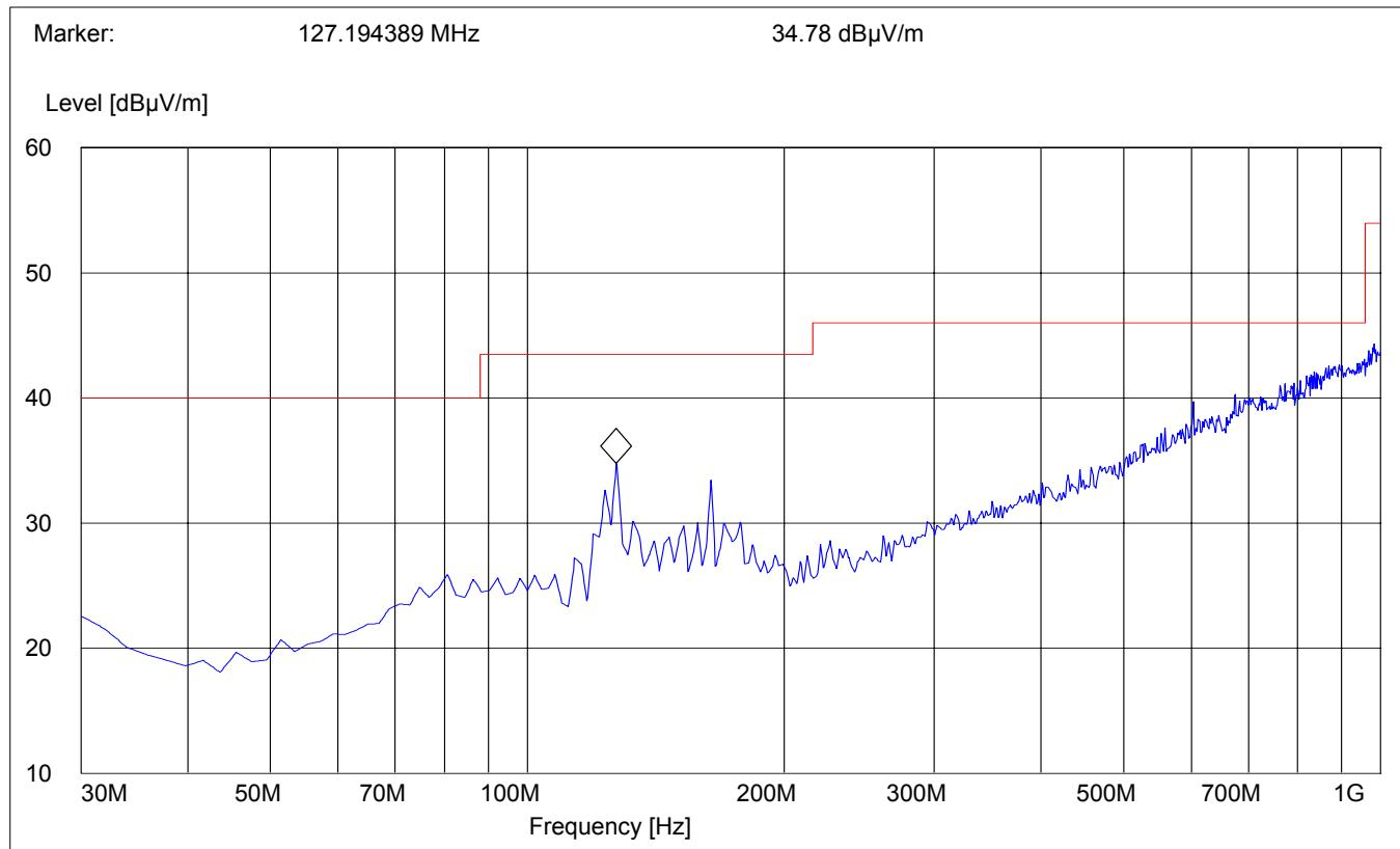
**EMISSION LIMITATIONS - Radiated (Transmitter)****§ 15.247 (c) (1)****Operating Mode: BT @ CH 0 + WLAN @ CH 1**
