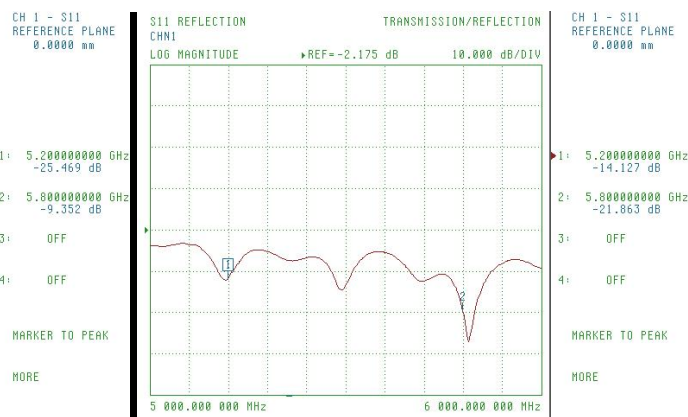
Return loss with 4.4mm separator
