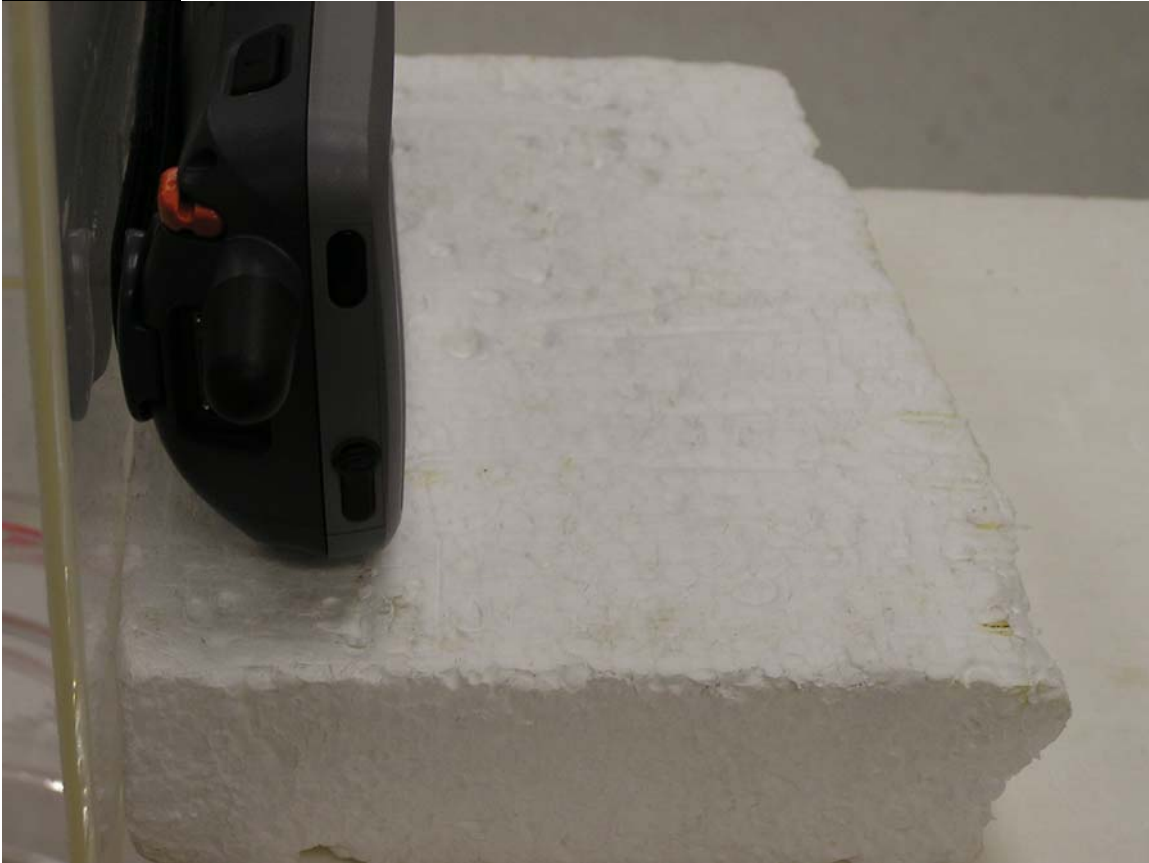
Photo 3 Belt clip touching phantom.
