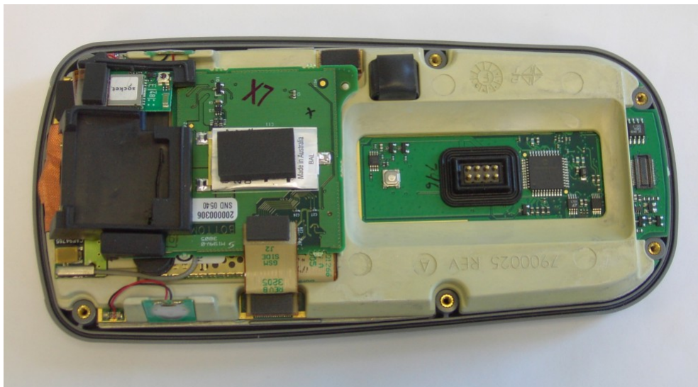
7900 “BUPE” Radio Placement Internal
