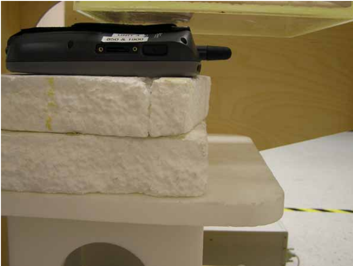
Photo 7 Belt clip touching phantom.
