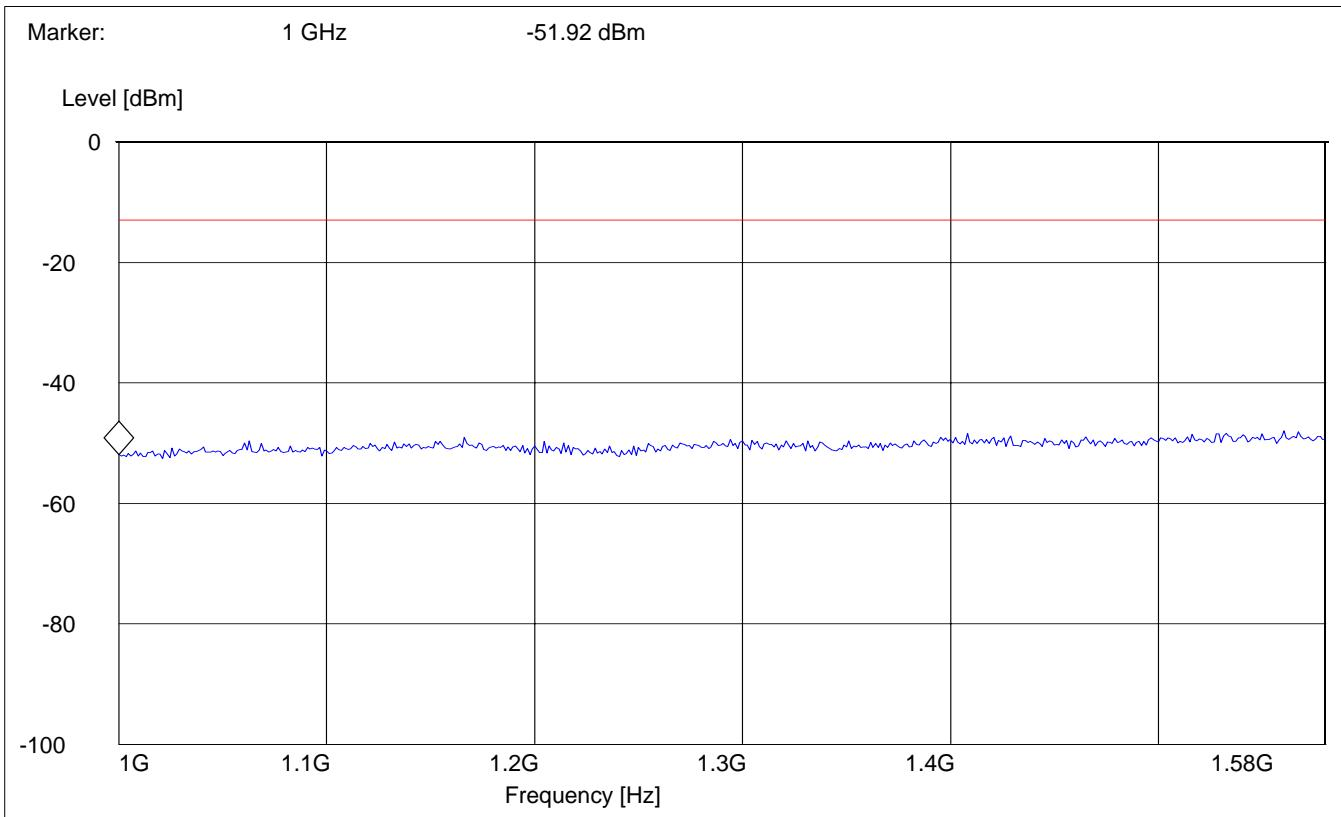
**RADIATED SPURIOUS EMISSIONS (GSM-850)****Tx @ 848.8MHz: 1.58GHz – 3GHz**
