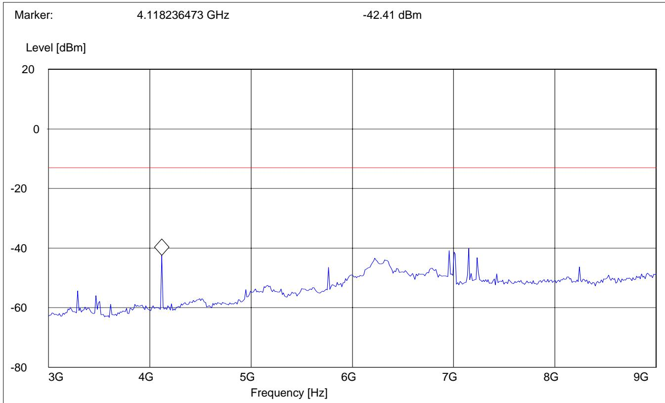
**RADIATED SPURIOUS EMISSIONS (GSM-850)****Tx @ 836.6MHz: 1GHz – 1.58GHz**
