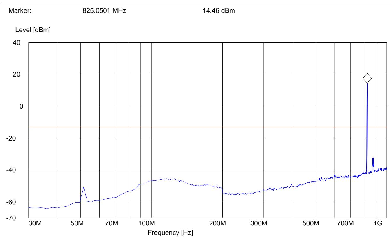
**RADIATED SPURIOUS EMISSIONS (GSM-850)****30MHz - 1GHz**
