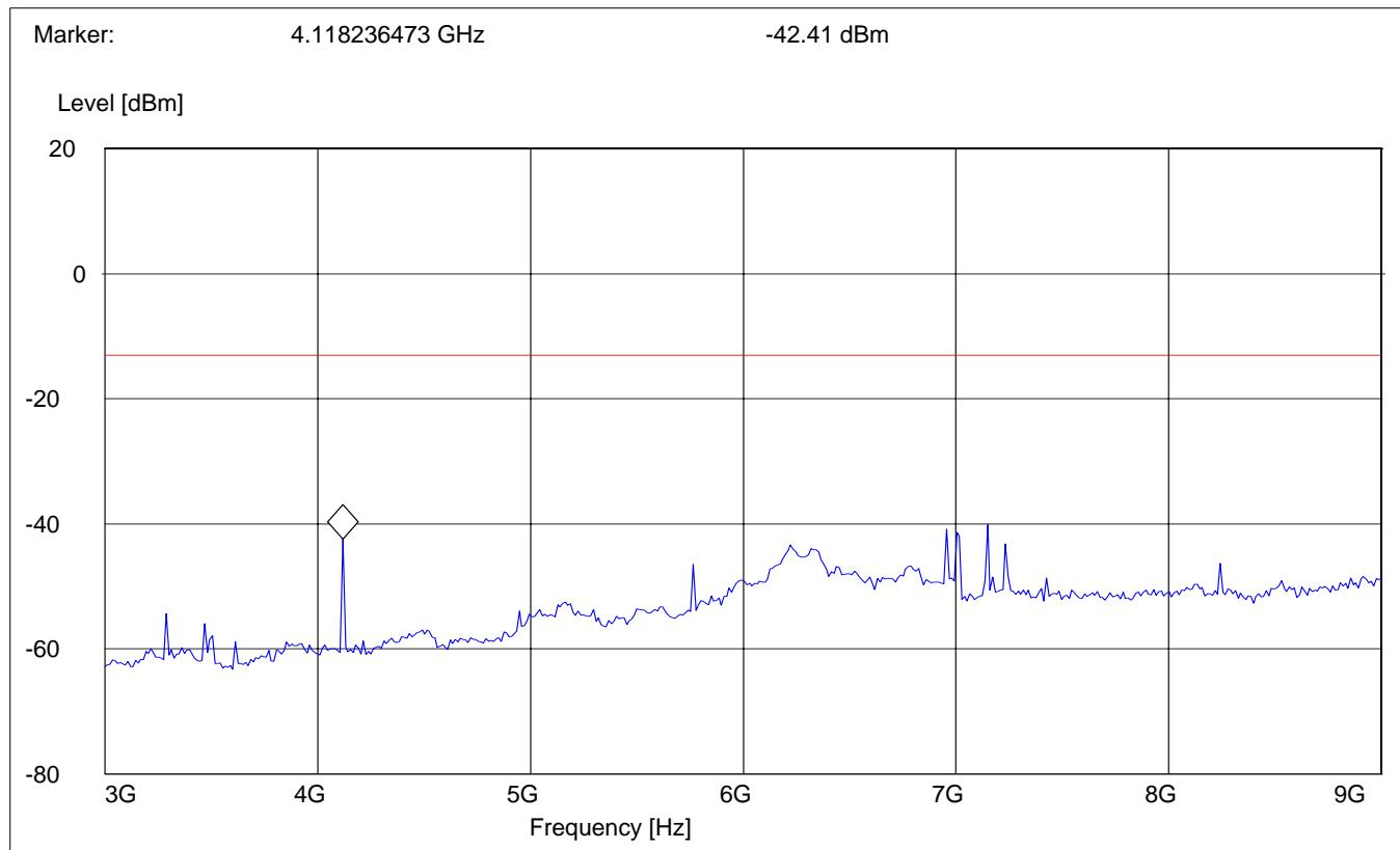
**RADIATED SPURIOUS EMISSIONS (GSM-850)****Tx @ 848.8MHz: 1GHz – 1.58GHz**
