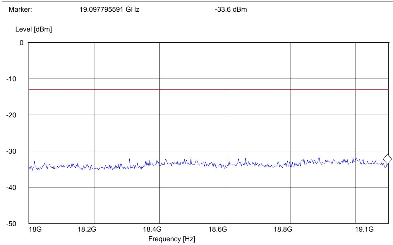
**RADIATED SPURIOUS EMISSIONS****18GHz – 19.1GHz**
