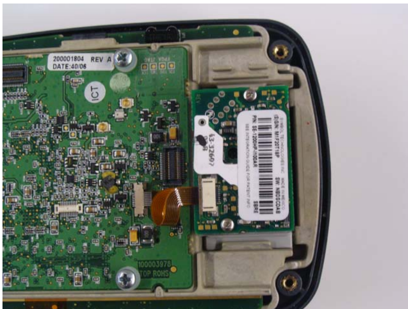
Close-up of SE 1200 engine placement in terminal
