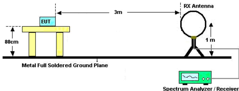
For radiated emissions from 30MHz to 1GHz
