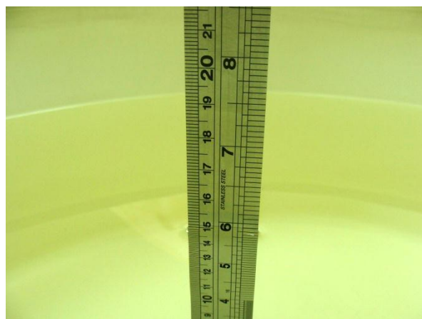
Fig 6.2 Photo of Liquid Height for Body SAR
