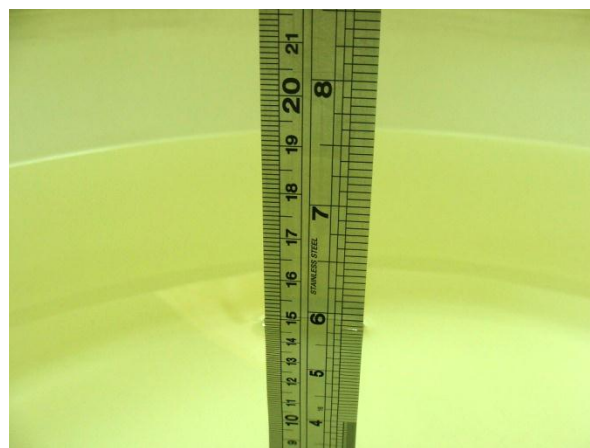
Fig 6.2 Photo of Liquid Height for Body SAR
