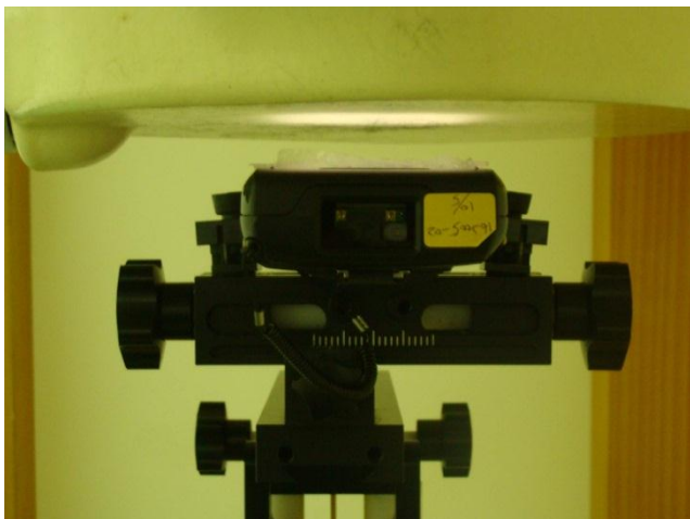
Front of the DUT and Battery 1 with 1.5 cm Gap
