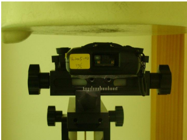
Back of the DUT and Battery 2 with 1.5 cm Gap
