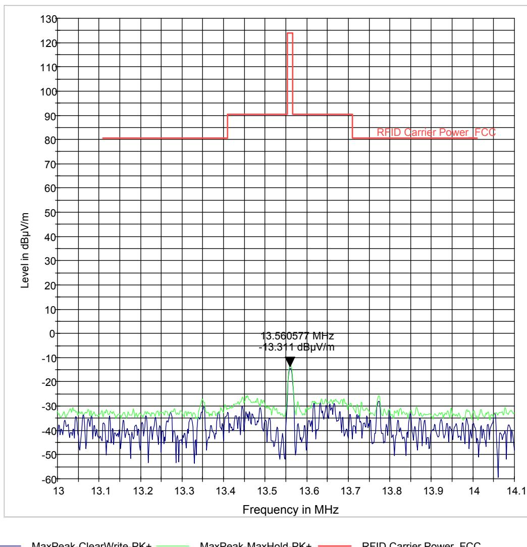
The red colored line shows the limit per part 15.225 extrapolated to 3m distance according to 15.31(f)(2), i.e. 40dB/decade.
