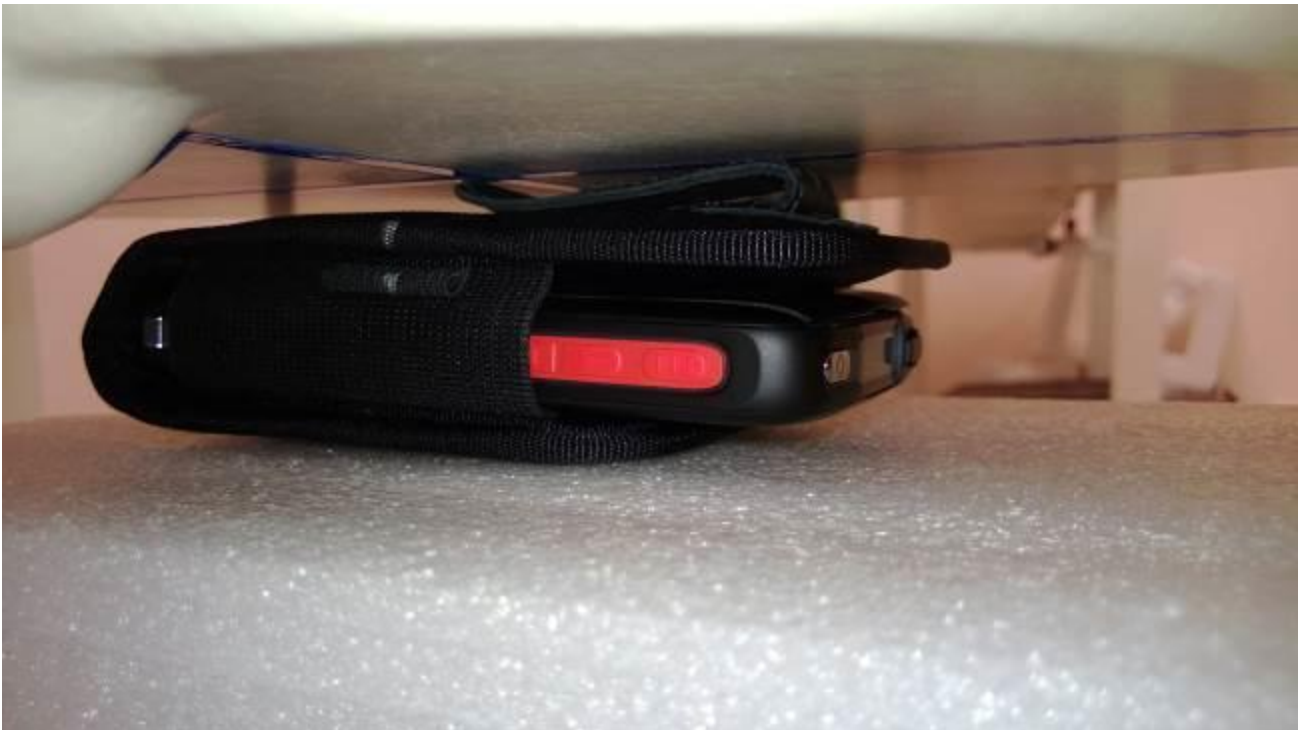
Photo 12: Back of EUT in Holster A at 0mm (Standard Battery)
