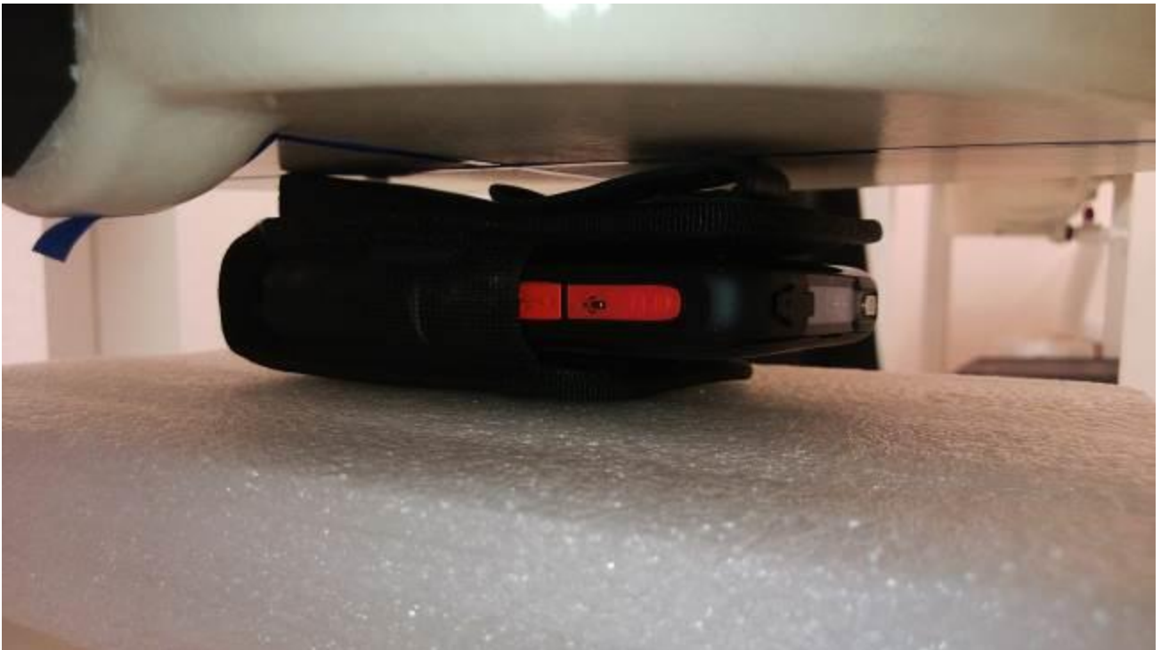
Photo 10: Front of EUT in Holster-1 at 0mm (Standard Battery)
