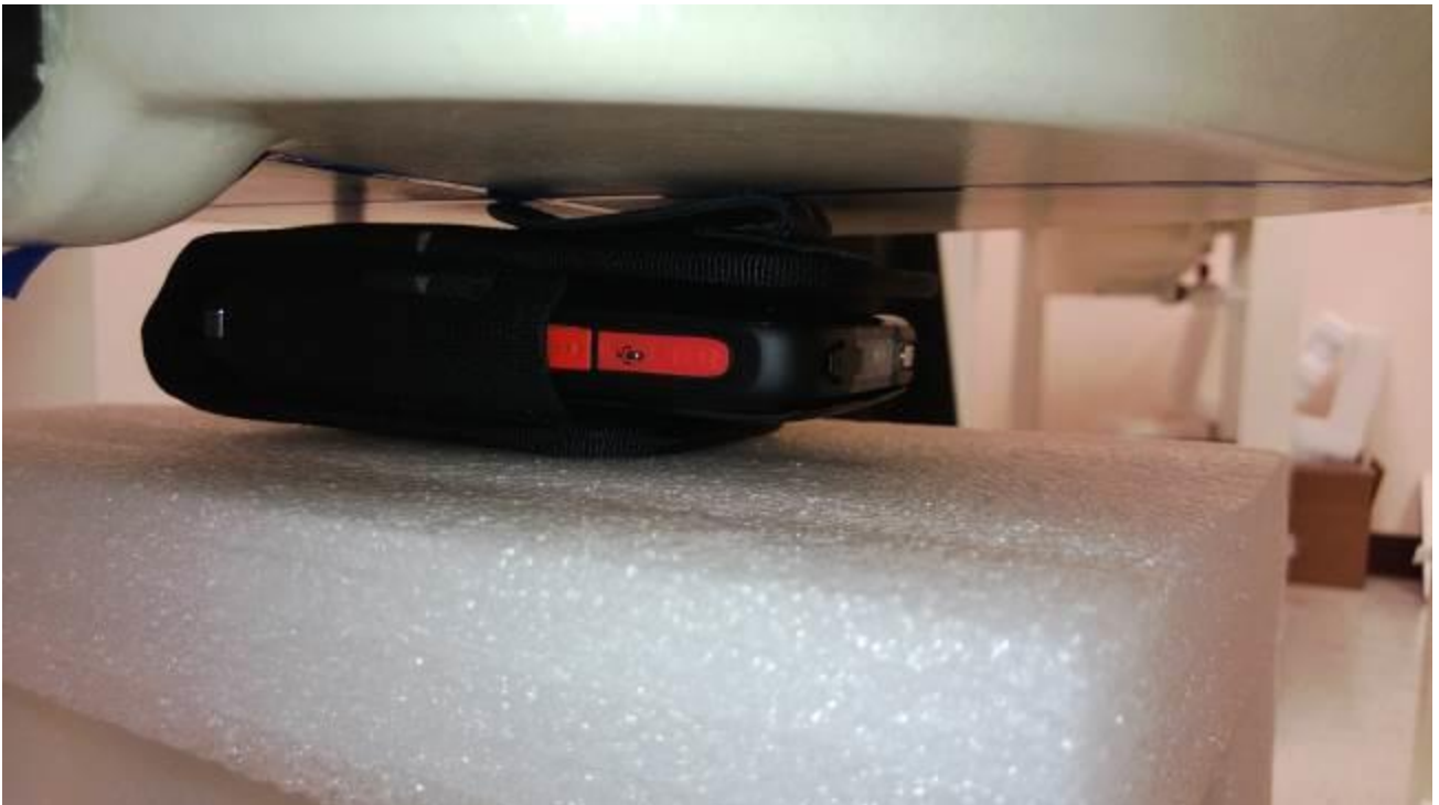
Photo 8: Front of EUT in Holster A at 0mm (Standard Battery)
