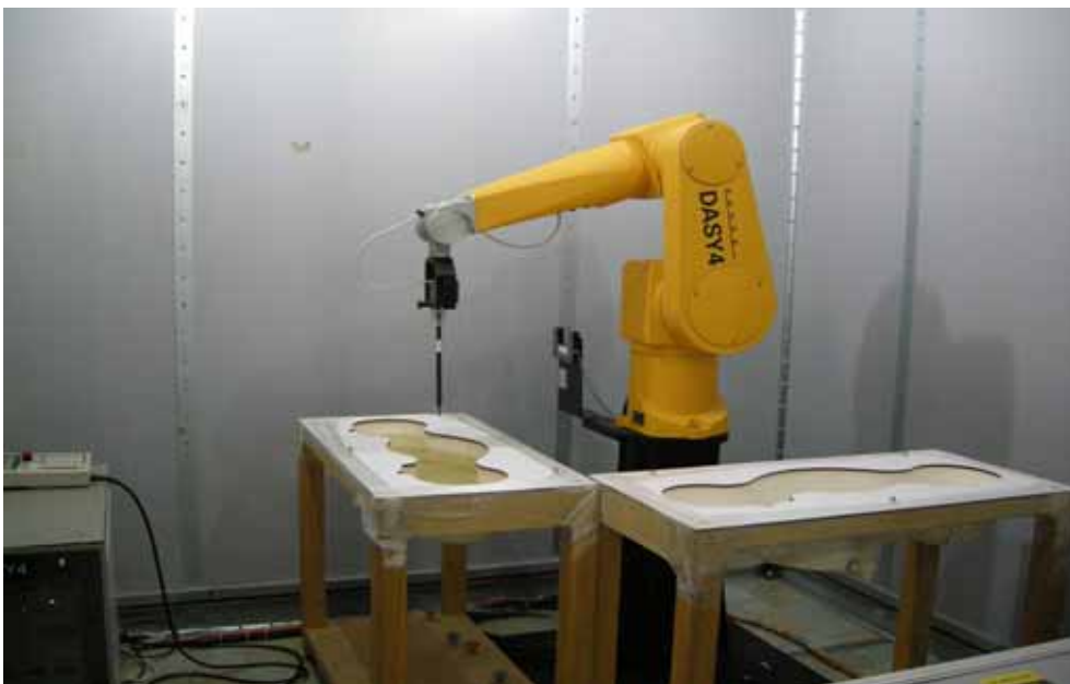
Fig. 4.1 SAR Measurement System
