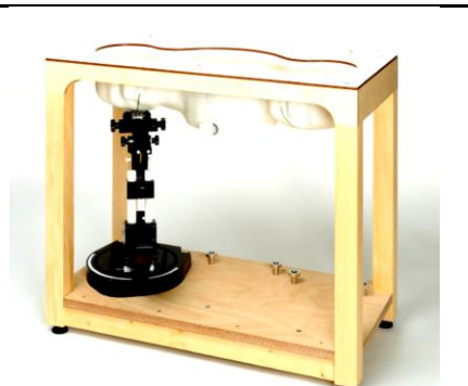
Fig 5.8 Photo of SAM Phantom
