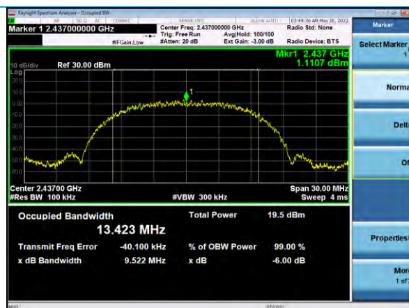
6 dB Bandwidth, Channel 6, 802.11b, 11Mbps
