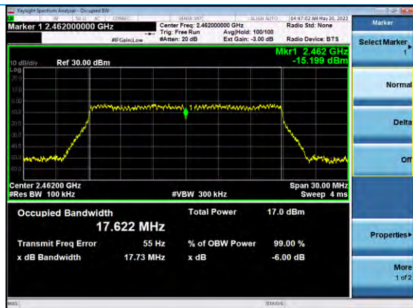
6 dB Bandwidth, Channel 11, 802.11n, MCS7
