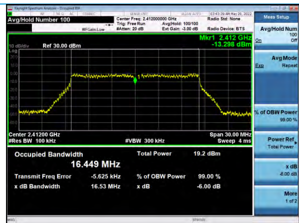
6 dB Bandwidth, Channel 1, 802.11g, 54Mbps
