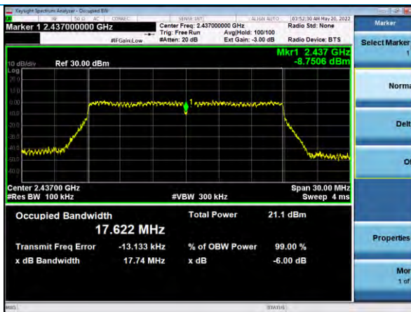
6 dB Bandwidth, Channel 6, 802.11n, MCS7
