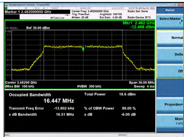
6 dB Bandwidth, Channel 11, 802.11g, 54Mbps
