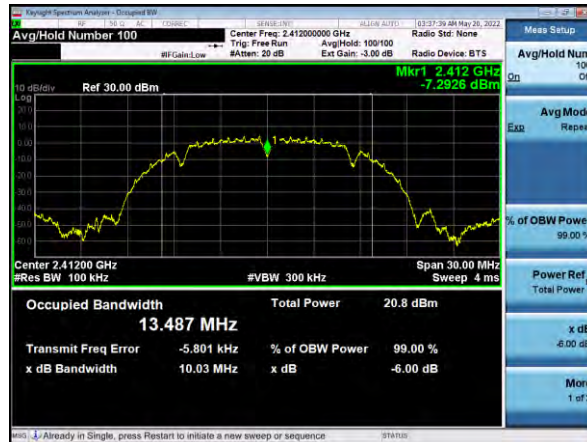
6 dB Bandwidth, Channel 1, 802.11b, 1Mbps
