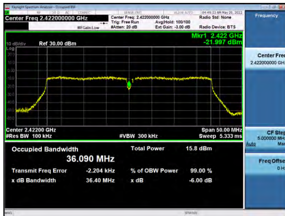
6 dB Bandwidth, Channel 3, 802.11n (40), MCS0
