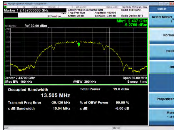
6 dB Bandwidth, Channel 6, 802.11b, 1 Mbps
