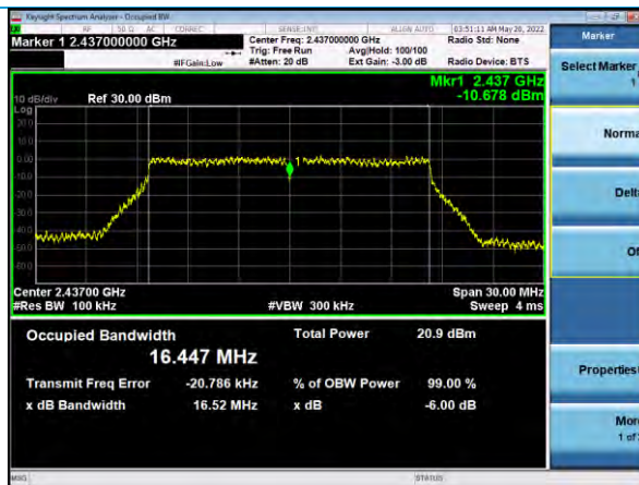
6 dB Bandwidth, Channel 6, 802.11g, 54Mbps
