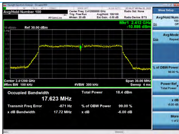
6 dB Bandwidth, Channel 1, 802.11n, MCS7
