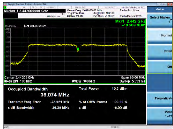
6 dB Bandwidth, Channel 7, 802.11n (40), MCS0
