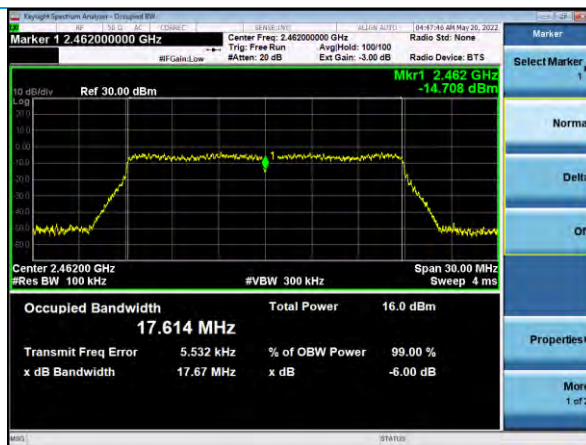
6 dB Bandwidth, Channel 11, 802.11n, MCS0
