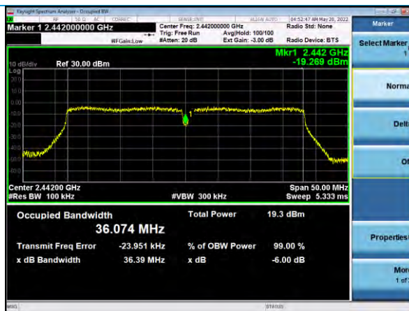
6 dB Bandwidth, Channel 3, 802.11n (40), MCS7
