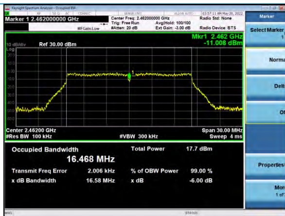
6 dB Bandwidth, Channel 11, 802.11g, 6Mbps
