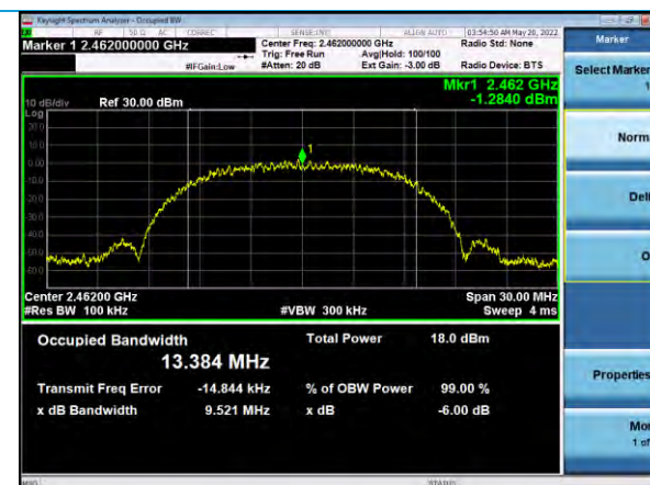
6 dB Bandwidth, Channel 11, 802.11b, 11Mbps
