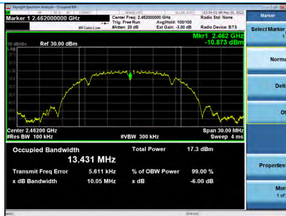
6 dB Bandwidth, Channel 11, 802.11b, 1Mbps
