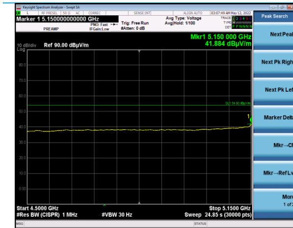
4500-5150 MHz, Horizontal Antenna, Average Channel 36, 802.11n MCS0 (20)
