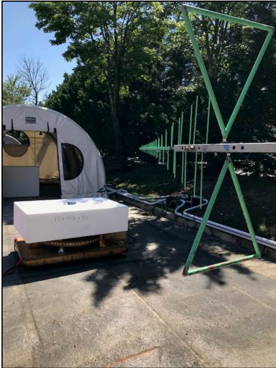
Photograph 3: Radiated Emissions Testing – Front View (Below 1 GHz)
