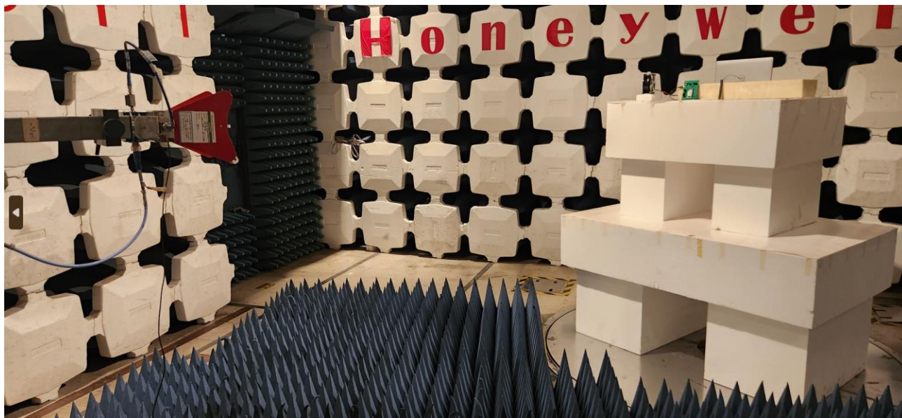
Radiated emission Test Setup – Horizontal Polarization
