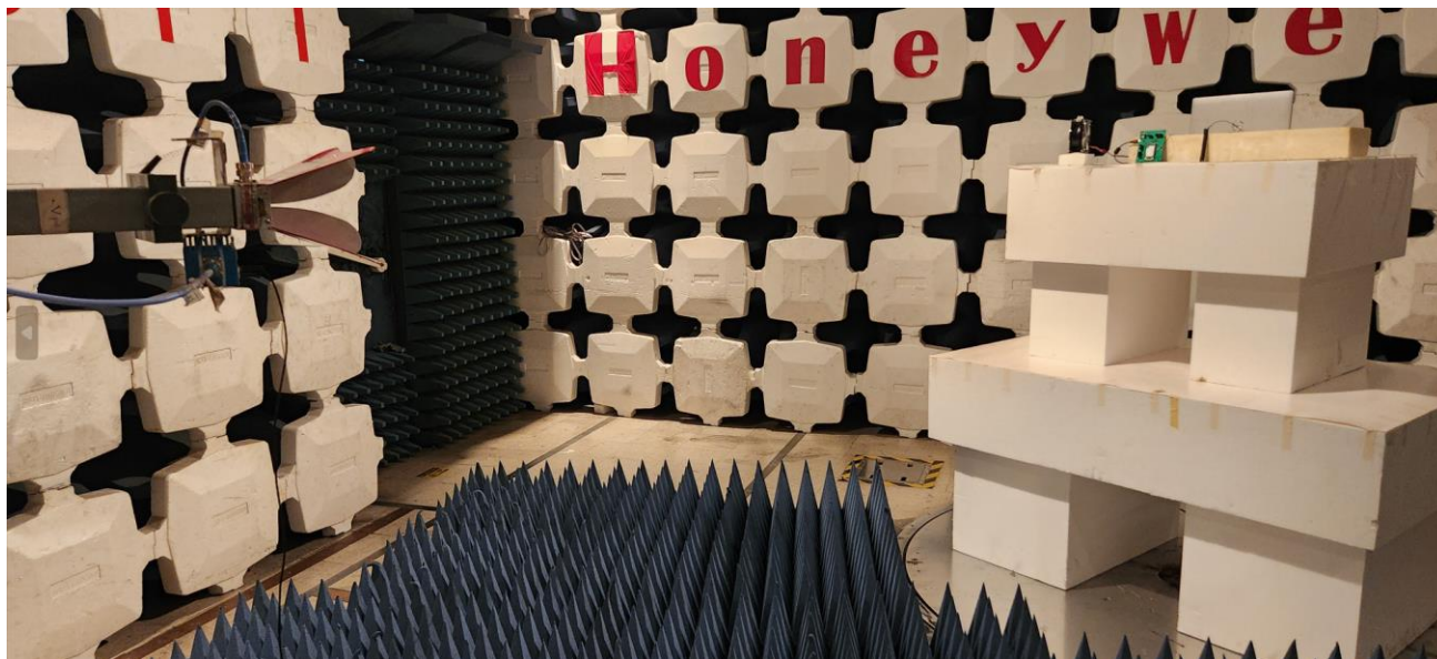
Radiated emission Test Setup – Vertical Polarization
