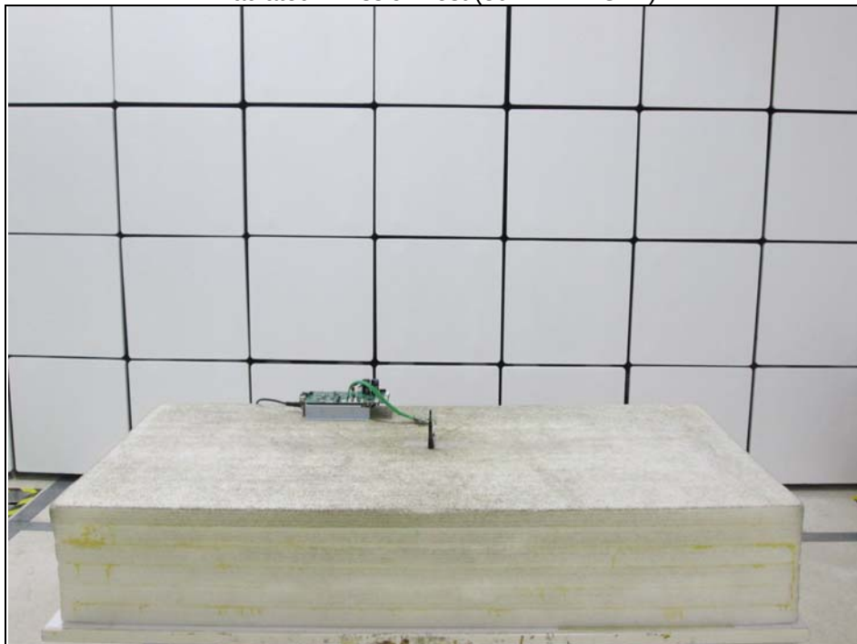
Radiated Emission Test (30MHz ~ 1GHz)
