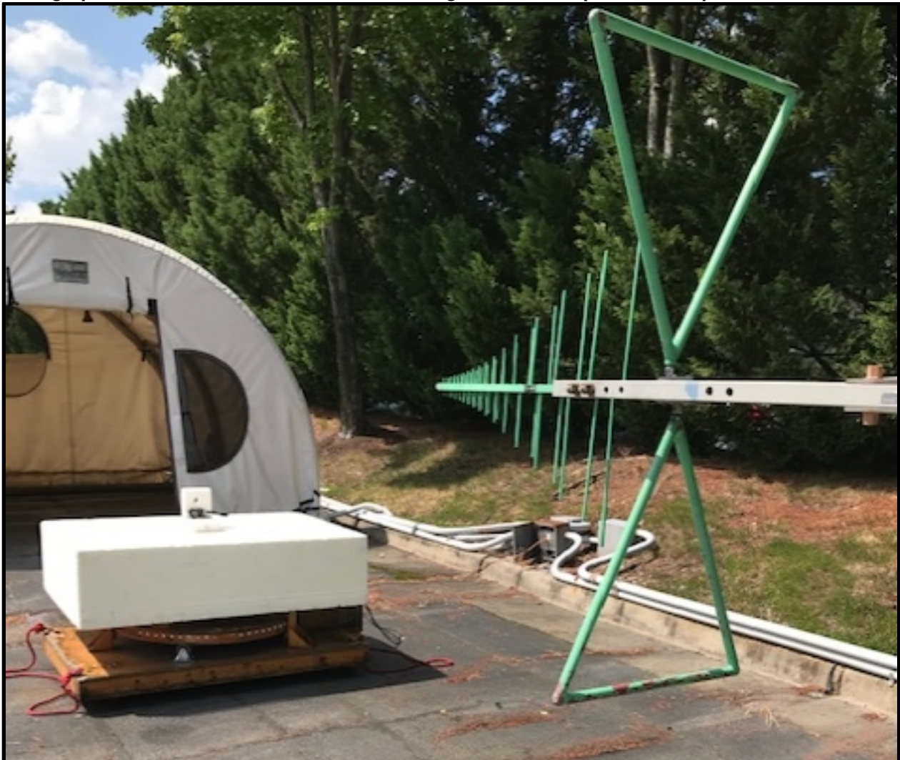
Photograph 2: Radiated Emissions Testing – Front View (Below 1 GHz)
