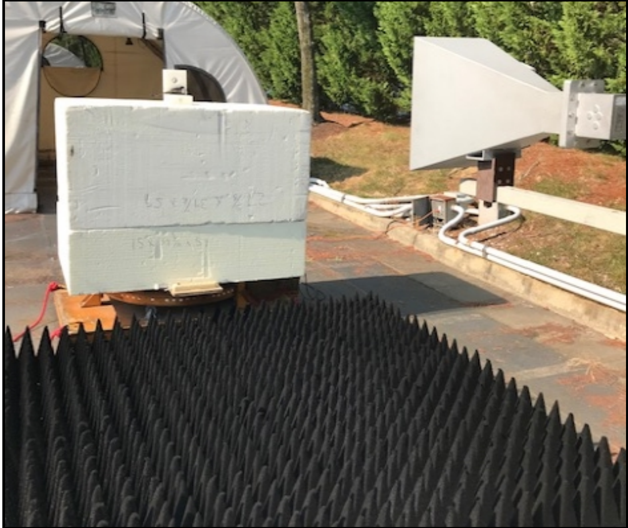
Photograph 1: Radiated Emissions Testing – Front View (Above 1 GHz)
