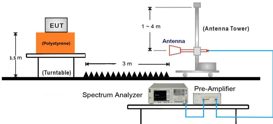
18GHz ~25GHz Test Setup:
