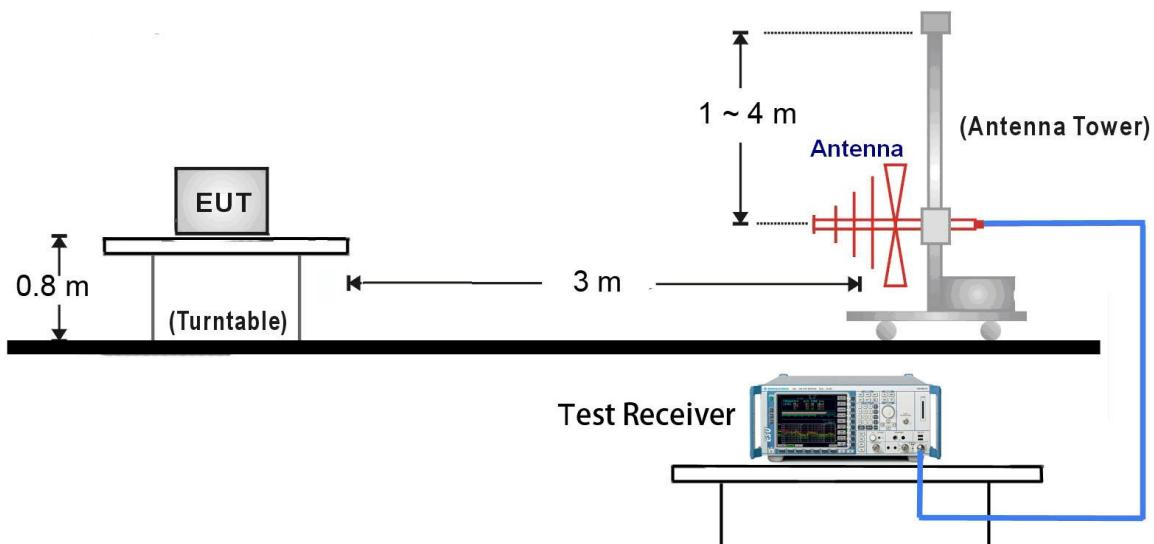
1GHz ~ 18GHz Test Setup:
