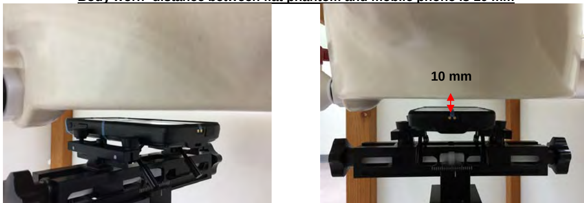
Fig.7 EUT Front side to flat phantom
