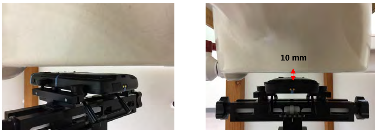
Fig.8 EUT Back side to flat phantom
