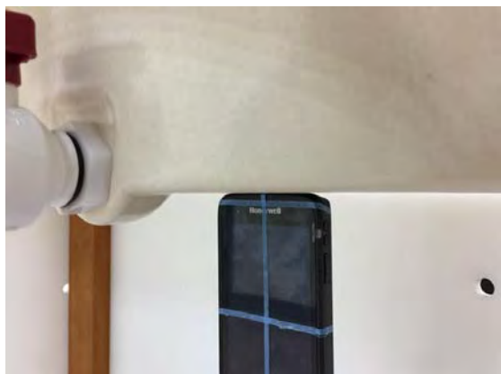
Fig.11 EUT Top side to flat phantom
