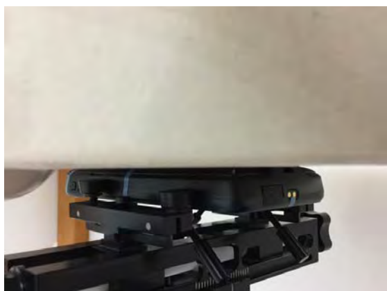
Fig.10 EUT Back side to flat phantom
