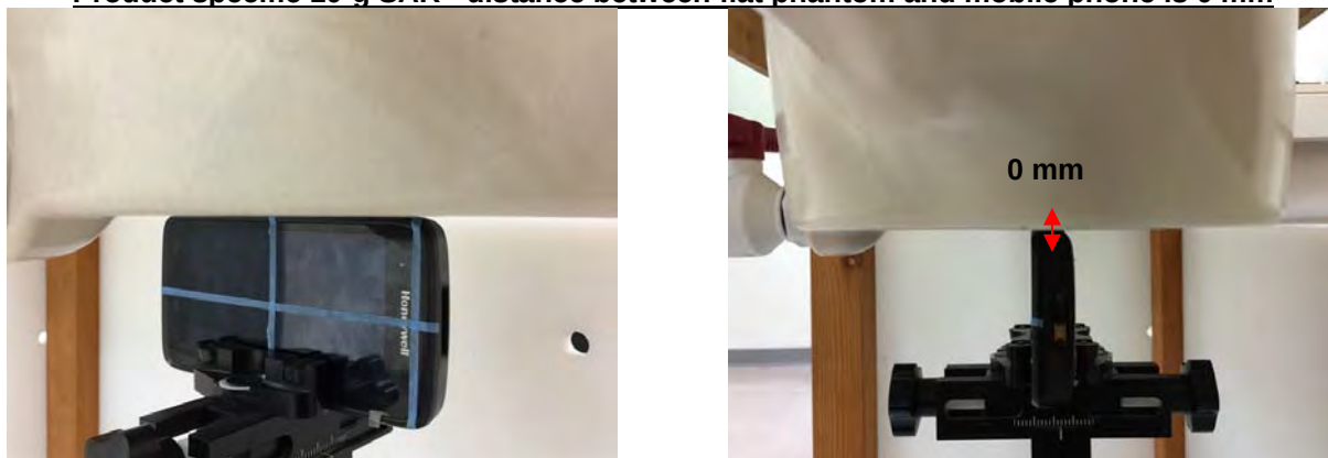
Fig.12 EUT Left side to flat phantom
