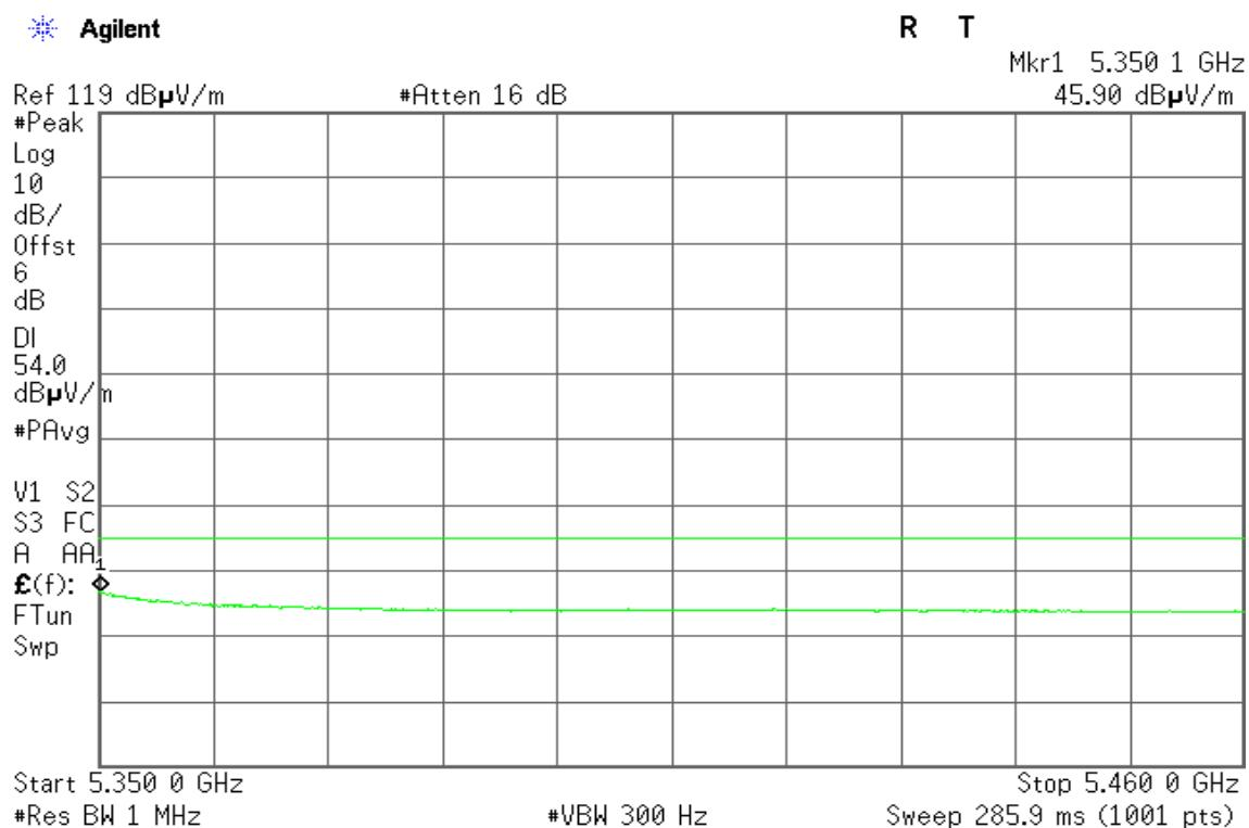
**Detector mode: Peak****Polarity: Horizontal**
