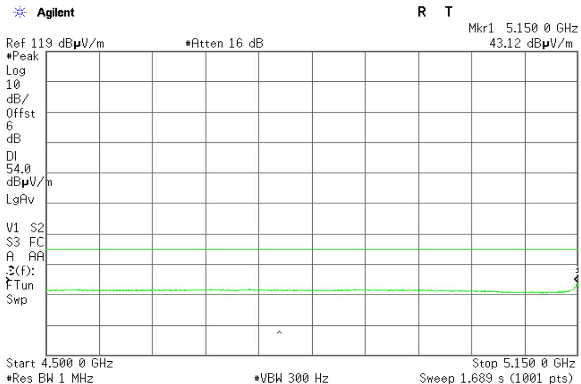
**Band Edges (IEEE 802.11a mode / 5320 MHz)****Detector mode: Peak****Polarity: Vertical**
