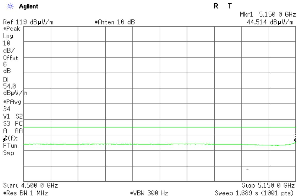
**Band Edges (IEEE 802.11a mode / 5320 MHz)****Detector mode: Peak****Polarity: Vertical**
