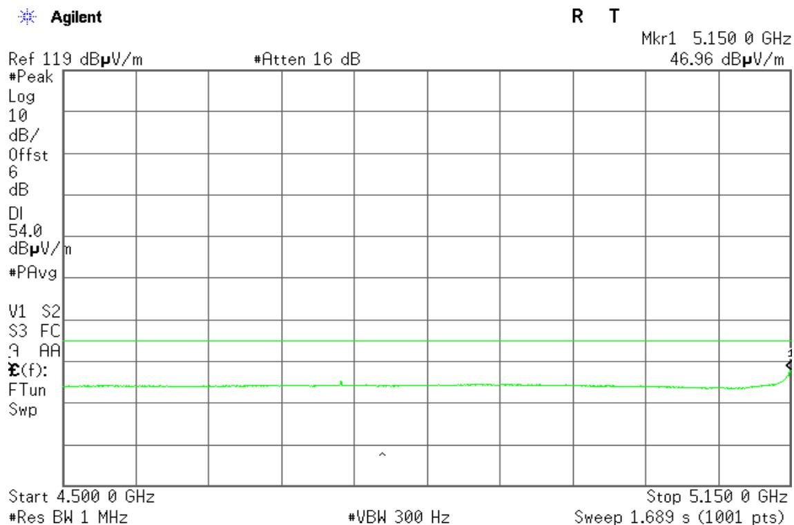
**Band Edges (IEEE 802.11a mode / 5320 MHz)****Detector mode: Peak****Polarity: Vertical**
