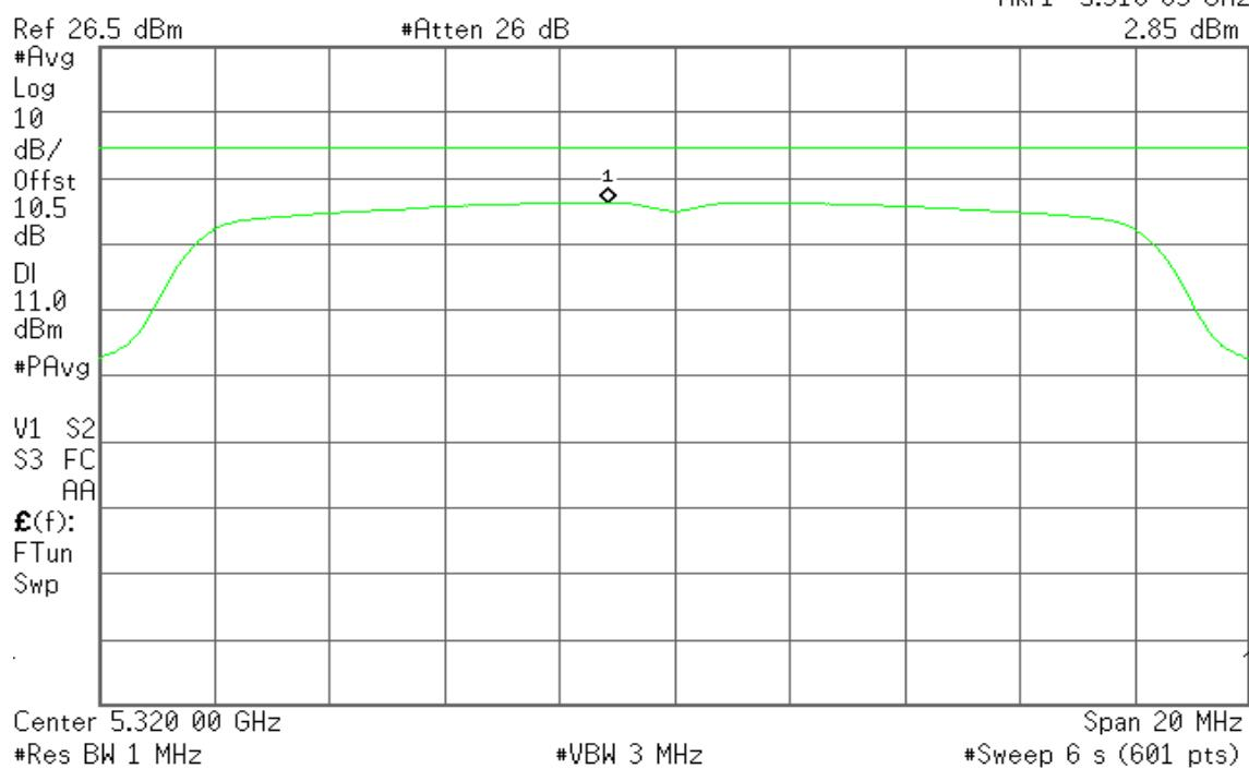
**IEEE 802.11n HT 20 MHz Channel mode / 5260 ~ 5320MHz****CH Low**
