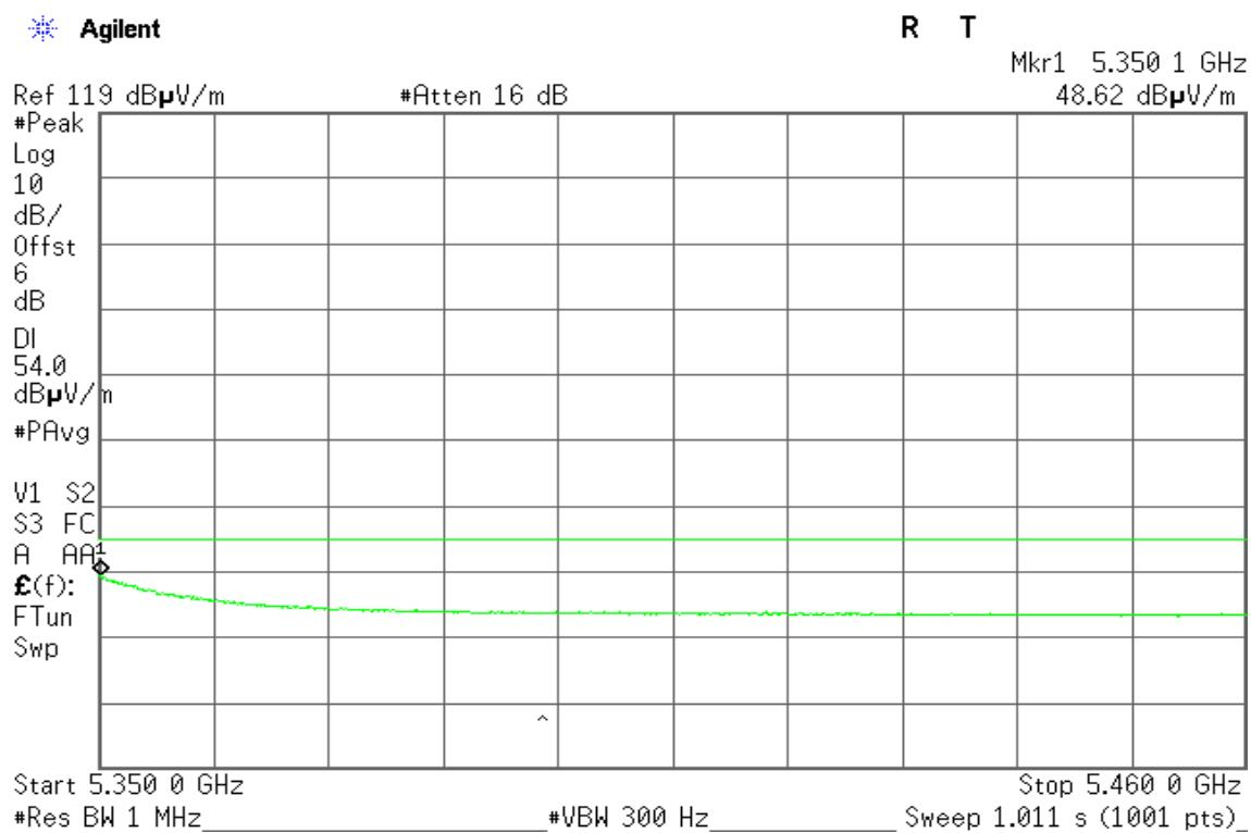
**Detector mode: Peak****Polarity: Horizontal**
