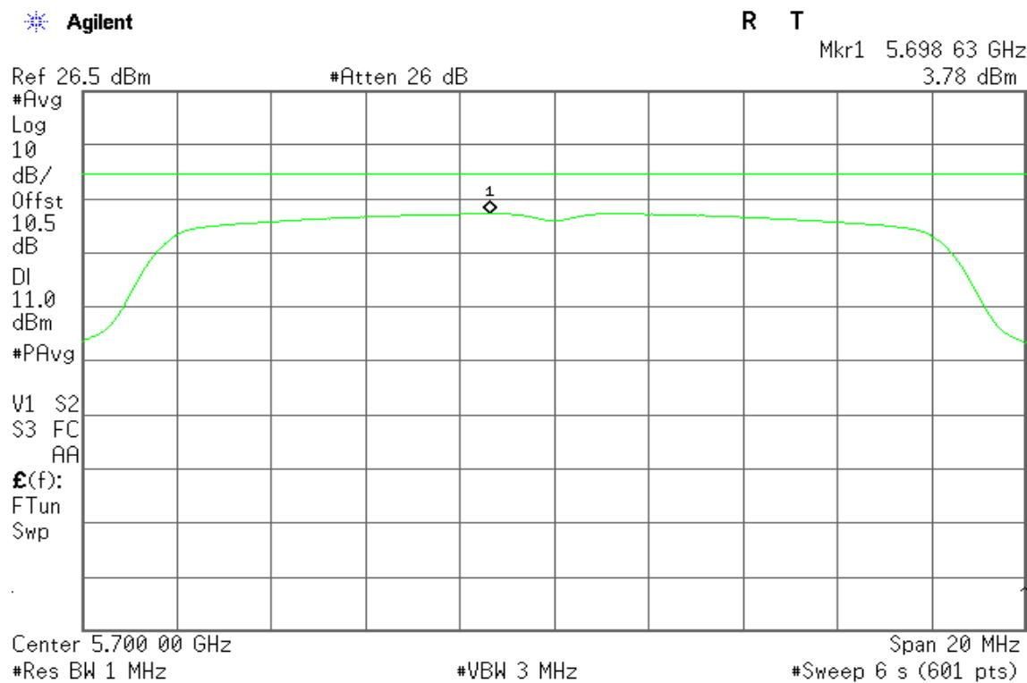
**IEEE 802.11n HT 20 MHz Channel mode / 5500 ~ 5700MHz****CH Low**
