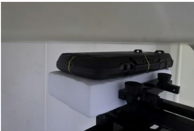
Rear Face, Test Separation 10 mm
