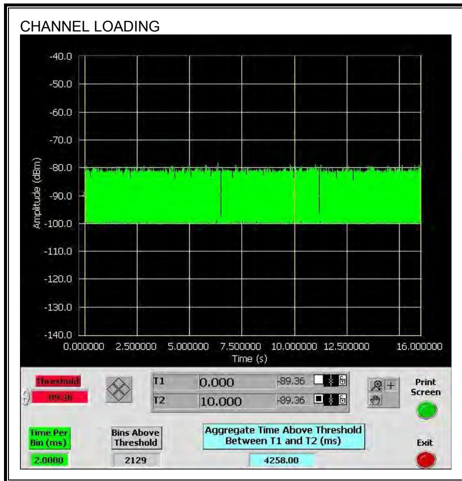
The level of traffic loading on the channel by the EUT is 42.58%
