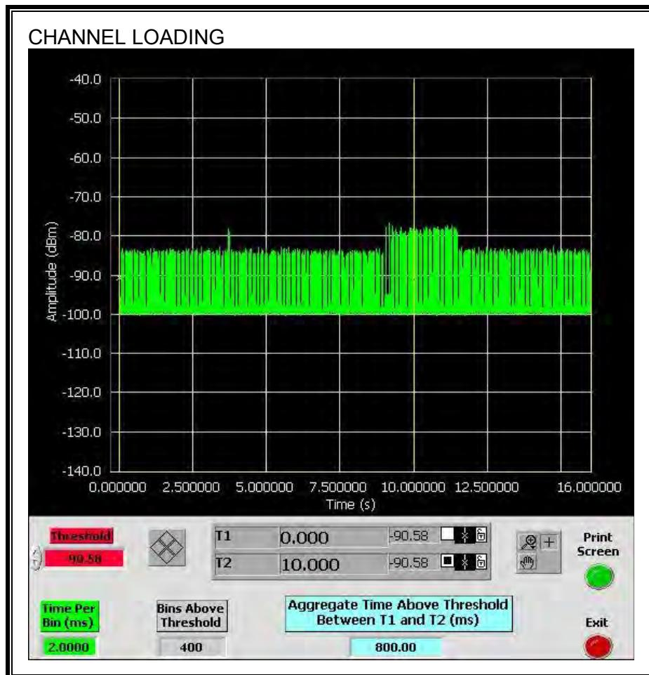
The level of traffic loading on the channel by the EUT is 8%
