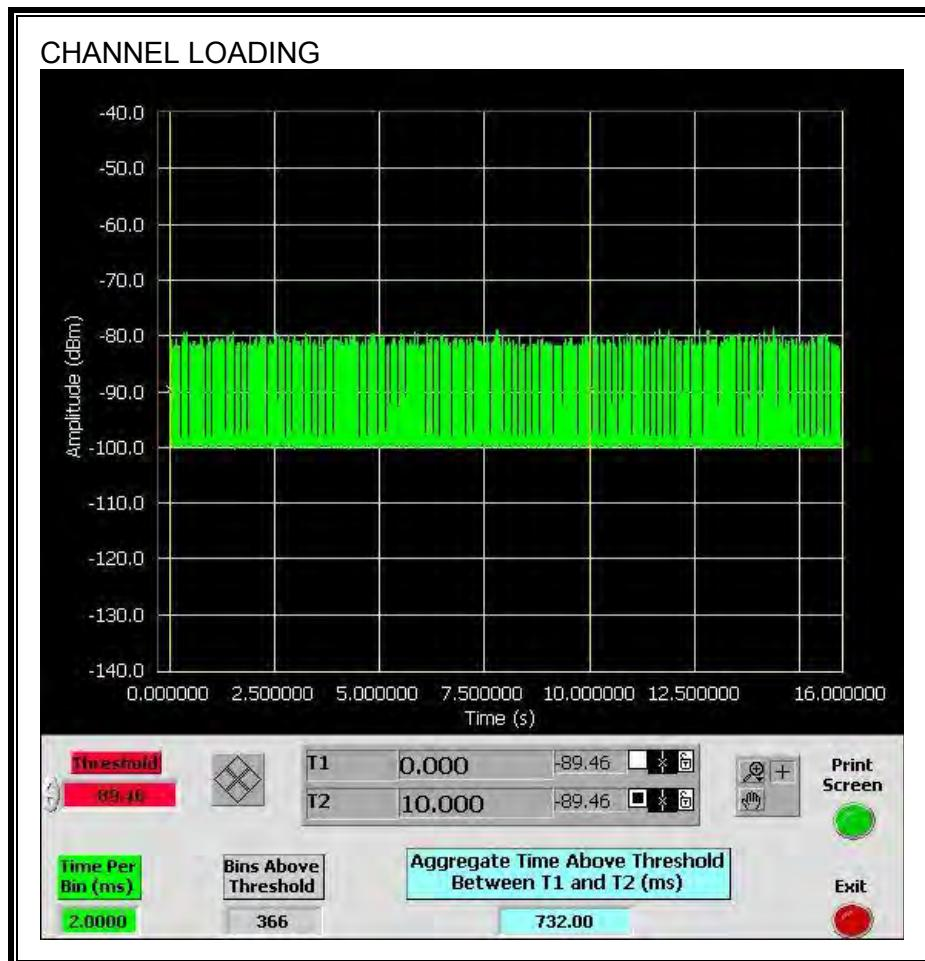
The level of traffic loading on the channel by the EUT is 7.32%
