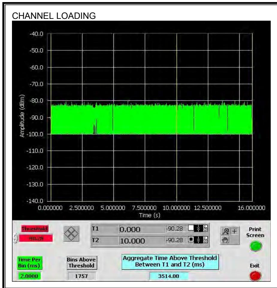
The level of traffic loading on the channel by the EUT is 35.14%
