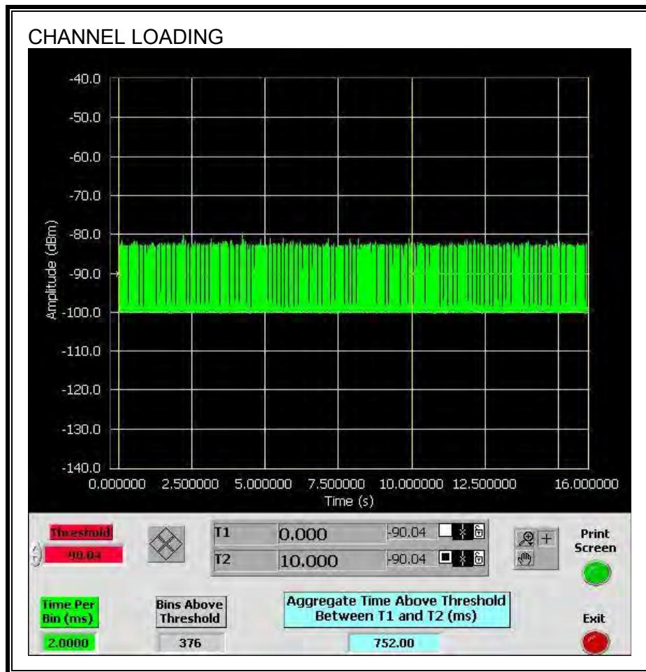
The level of traffic loading on the channel by the EUT is 7.52%
