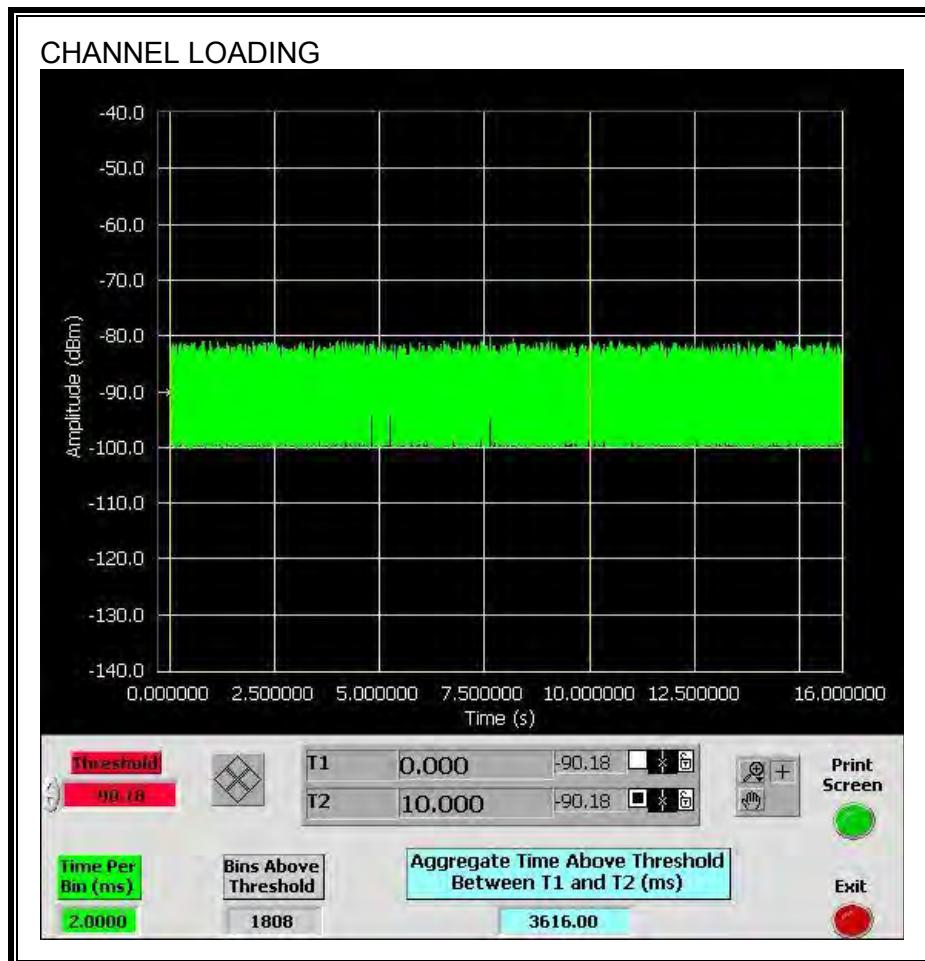
The level of traffic loading on the channel by the EUT is 36.16%
