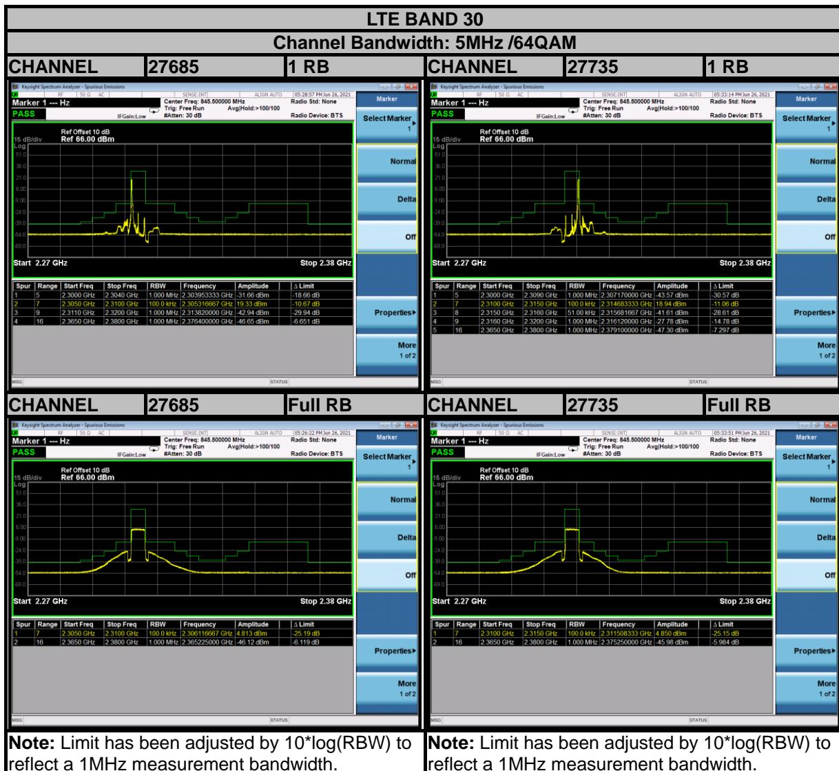
**Note:** Limit has been adjusted by  $10 \times \log(\text{RBW})$  to reflect a 1MHz measurement bandwidth.
