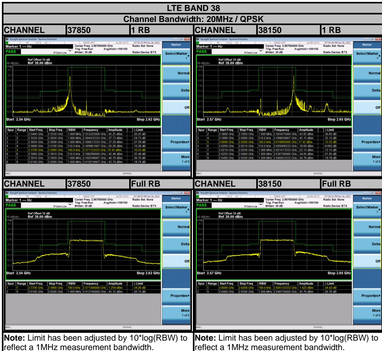
**Note:** Limit has been adjusted by  $10 \cdot \log(RBW)$  to reflect a 1MHz measurement bandwidth.
