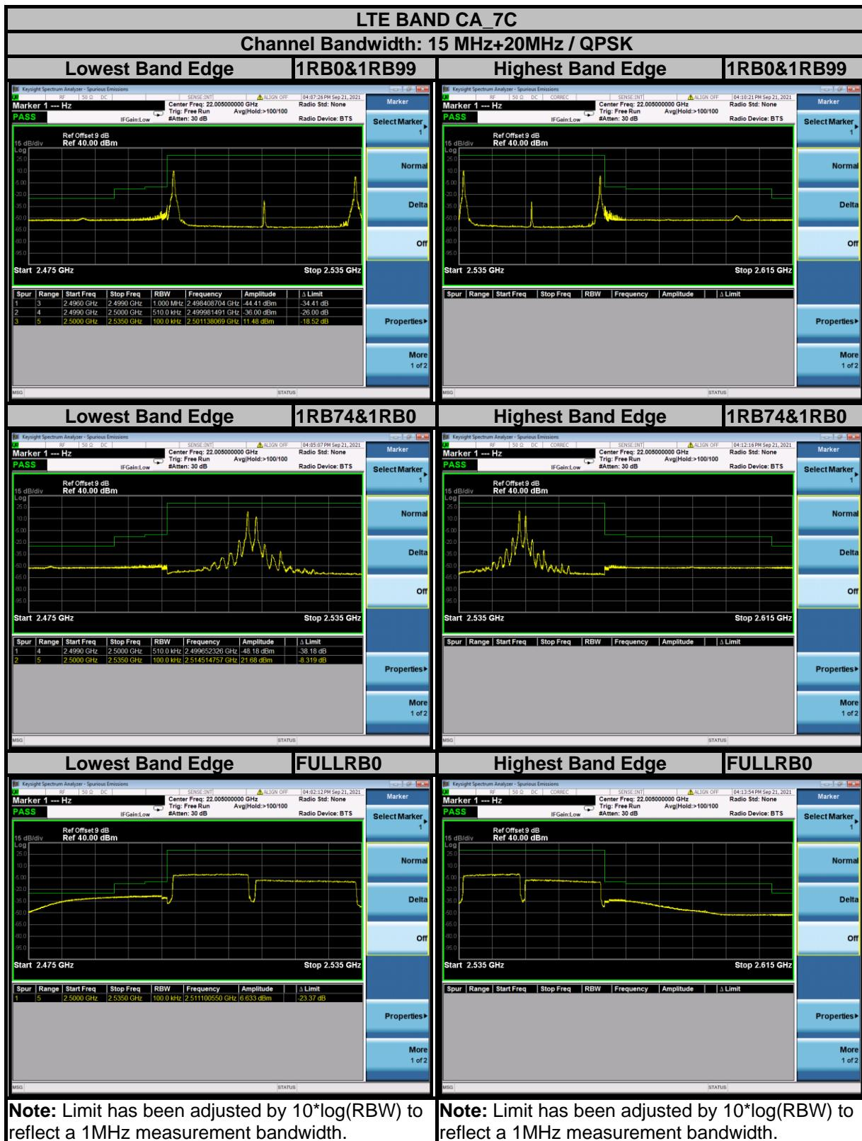
**Note:** Limit has been adjusted by  $10 \cdot \log(RBW)$  to reflect a 1MHz measurement bandwidth.
