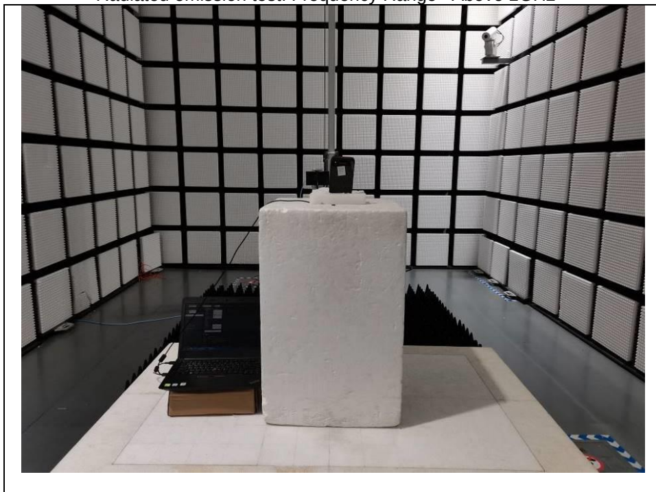
Radiated emission test: Frequency Range< Above 1GHz >
