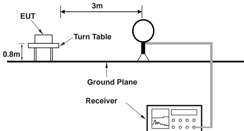
Setup diagram for Radiation(Below 1G) Test
