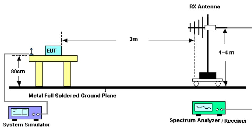
For radiated test above 1GHz
