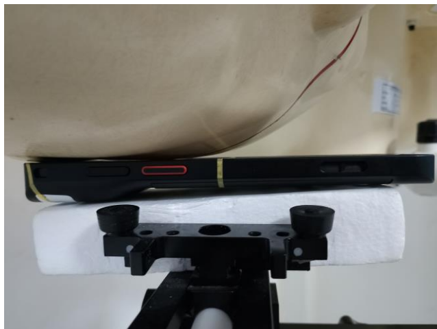
Right Cheek, Test Separation 0 mm
