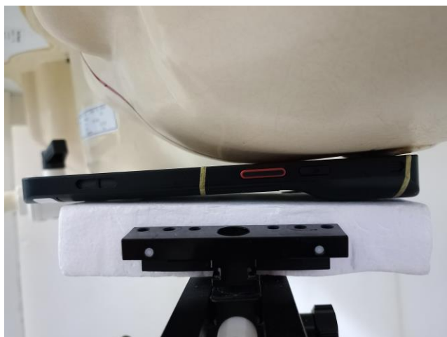
Left Cheek, Test Separation 0 mm
